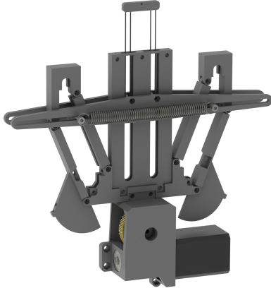
Fig. 15: The last iteration of the variable stiffness mechanism device without a rest length adjustment mechanism.
