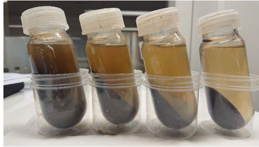
Figure 65 Resulting centrate from activated sludge samples pre-conditioning tests. From left to right, initial MLSS: 38, 30.4, 22.8, 15.2 g L -1 . Final MLSS: 1.14, 0.8, 0.67, 0.37 g L -1 .
