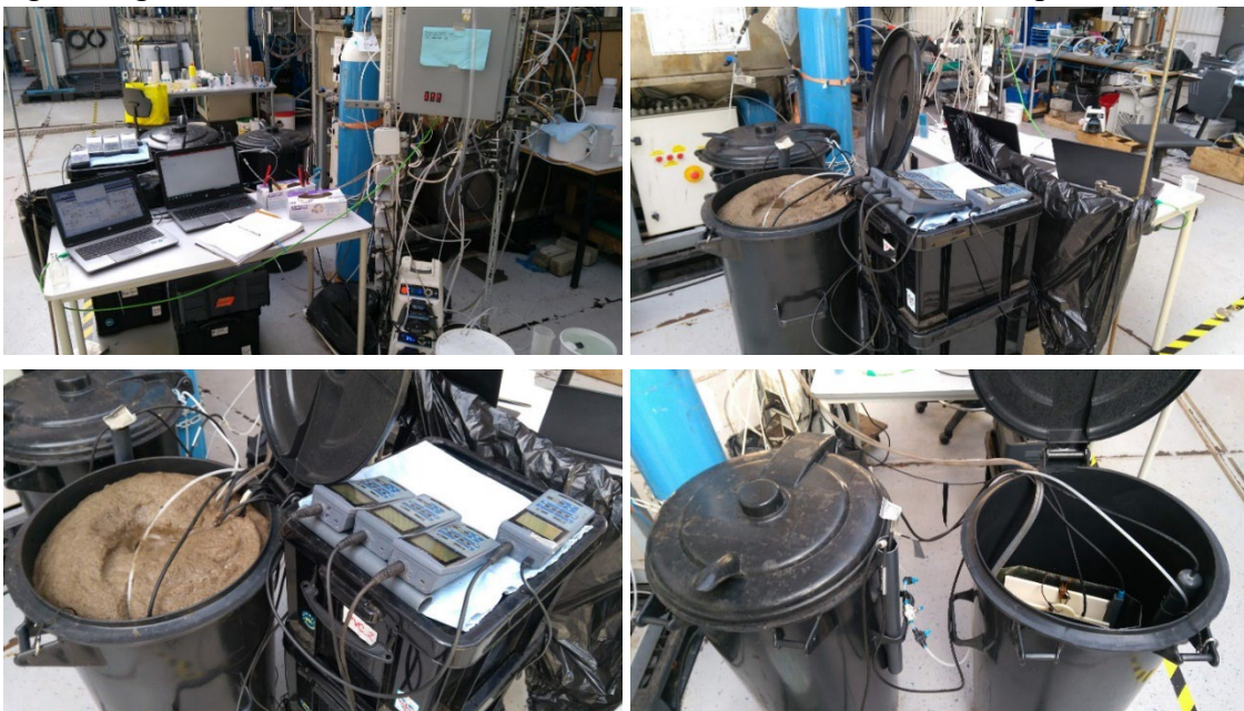
Figure 59 Experimental setup for testing the submerged membranes in high MLSS activated sludge.
