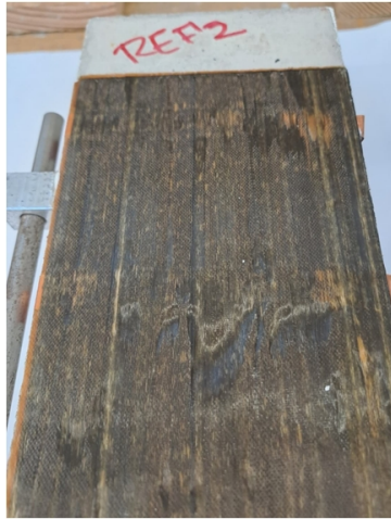
Figure 4.2: Indentations in REF 2 sample after curing
