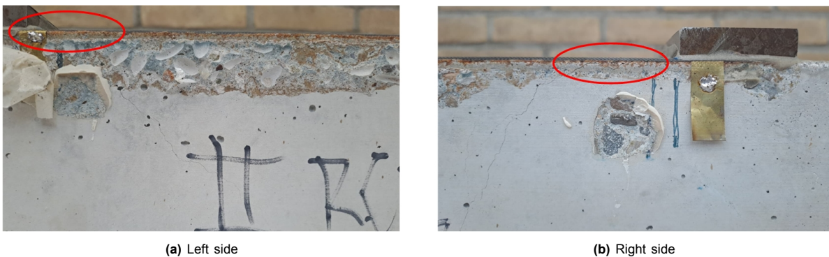
Figure 5.2: Post-test images of Specimen 2-REF3 showing delamination in the regions highlighted with red circles.
