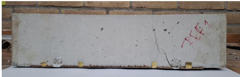
Figure D.1: Specimen REF1 after testing
