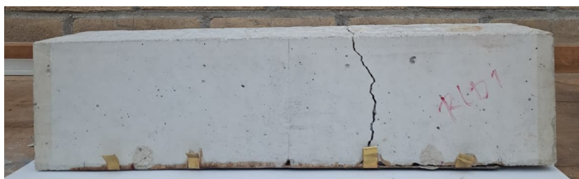
Figure D.4: Specimen RLD1 after testing
