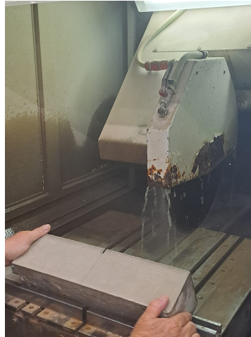
Figure 3.3: Creating notches in concrete beams using a diamond grinding disk
