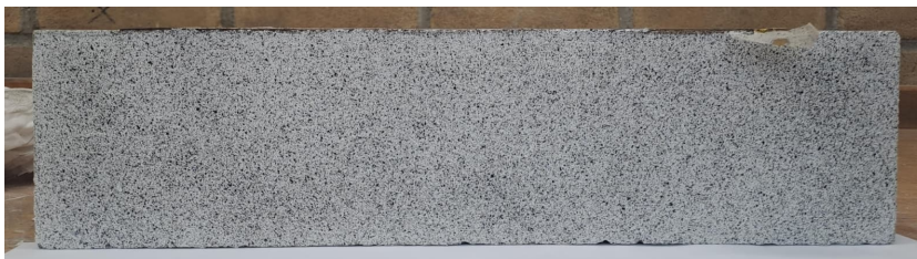
Figure 3.9: Stochastic pattern applied over the full length of the beam
