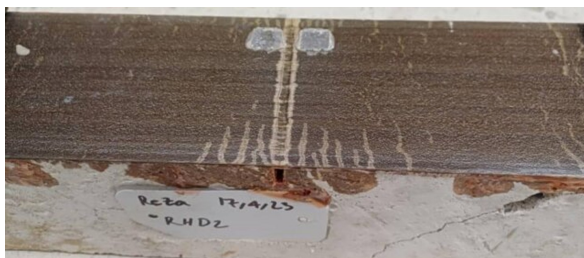
Figure 2.6: Mechanochromic effect on retrofitted concrete beam [7]
