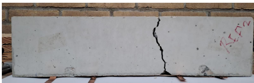
Figure D.2: Specimen REF2 after testing
