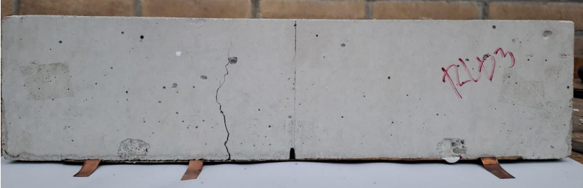
Figure D.6: Specimen RLD3 after testing
