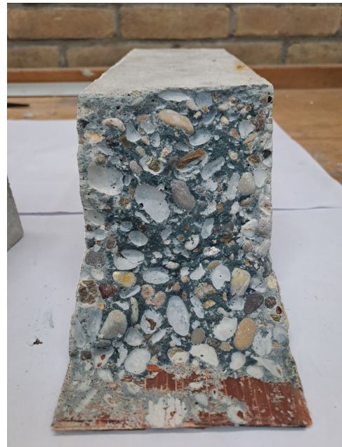
Figure 4.23: Cross section specimen 2-REF2 without glued support plates after testing
