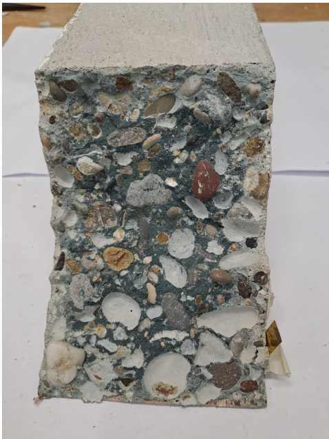
Figure 4.22: Cross section specimen 2-REF1 with glued support plates after testing
