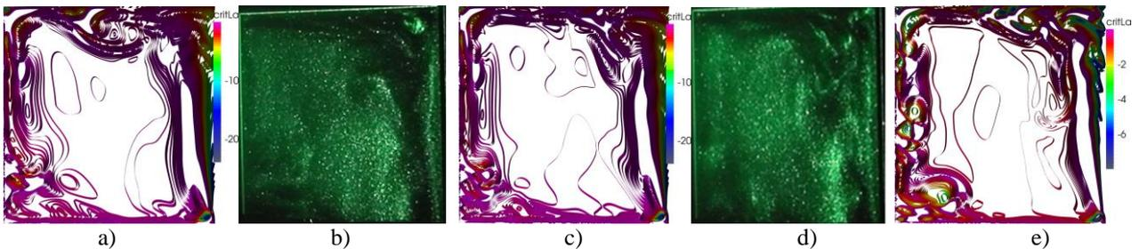
**Figure 3.** The meridian flow, a)  $Re=3925$ ,  $\lambda_2$  criterion, b)  $Re=3925$ , Kalliroscope, c)  $Re=4579$ ,  $\lambda_2$  criterion, d)  $4579$ , Kalliroscope, e)  $Re=7031$ ,  $\lambda_2$  criterion,  $\Gamma=1.04$ ,  $Rm=2.2$ , the inner cylinder (on the left) and the bottom disk rotate.
