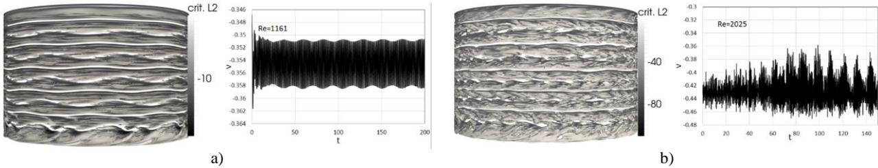
**Figure 1.** The flow structure and instability characteristics obtained for asymmetric end-walls boundary conditions, a)  $Re=1161$ , b)  $2025$ ,  $\Gamma=11.75$ ,  $Rm=19$ , the inner cylinder and the bottom disk rotate.
