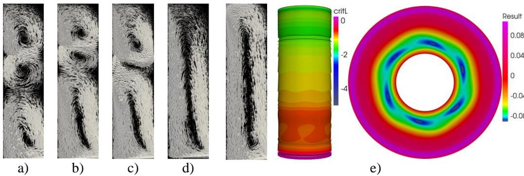
**Figure 2.** The meridian flow, a)  $Re=108$ , b)  $200$ , c)  $269.5$ , d)  $281.5$ , e)  $562.5$  – transition to unsteadiness, azimuthal section of the rotor boundary layer,  $z=-0.8149$ ,  $\Gamma=1.04$ ,  $Rm=2.2$ , the inner cylinder (on the left) and the bottom disk rotate.
