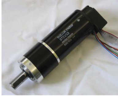
Figure 3.10: The PTO (motor, gearbox and encoder) [30]
