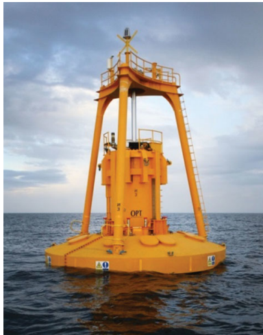
Figure 2.4: Ocean Power Technology's PowerBuoy, A point absorber [16]
