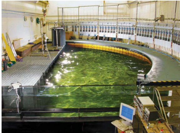
Figure 2.10: The Edinburgh curved wave tank
