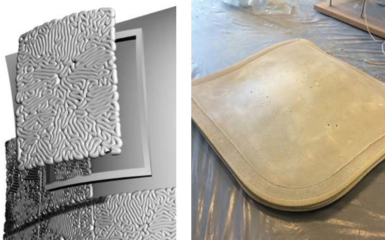
Figure 105 - Potential schemes for Fully-printed panels. [Left: facade Panels. Right: Printed with Edge perimeter] source: Author, 3TU Lighthouse 2016
