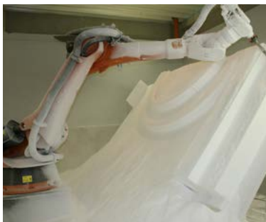
Figure 3 : Milling techniques can be used to generate complex free-form geometries. How viable is this for large-scale structures? source: accentform.com
