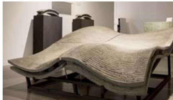
Figure 16: Manufacturing of free-form panels using concrete additive manufacturing. Note: surface finish exhibits layered texture source: Buswell et al. Lonborough university
