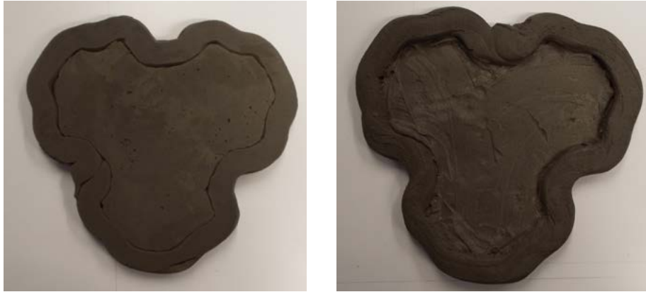
Figure 99 - Printed and cast panels. Note interface between printed and cast material source: Author
