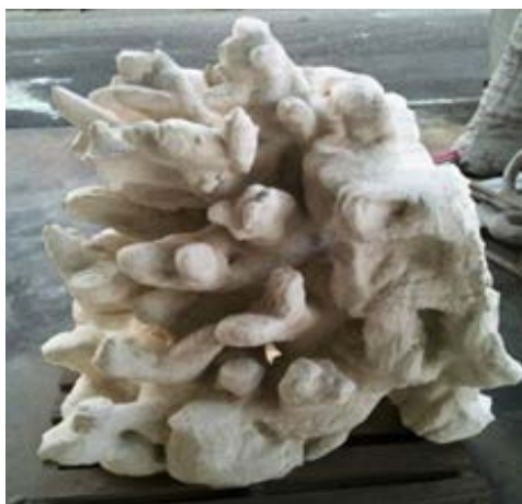
Figure 41 - D-Shape Printing Process used to construct artificial reef source: D-Shape.com
