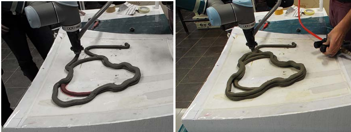
Figure 97 - Printing of stacked filaments source: Author
