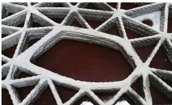
Figure 34: Use of multiple EPS Moulds to create rib-stiffened funicular floor system. The result is a neat and accurate geometry, however, is the manufacturing process efficient?
