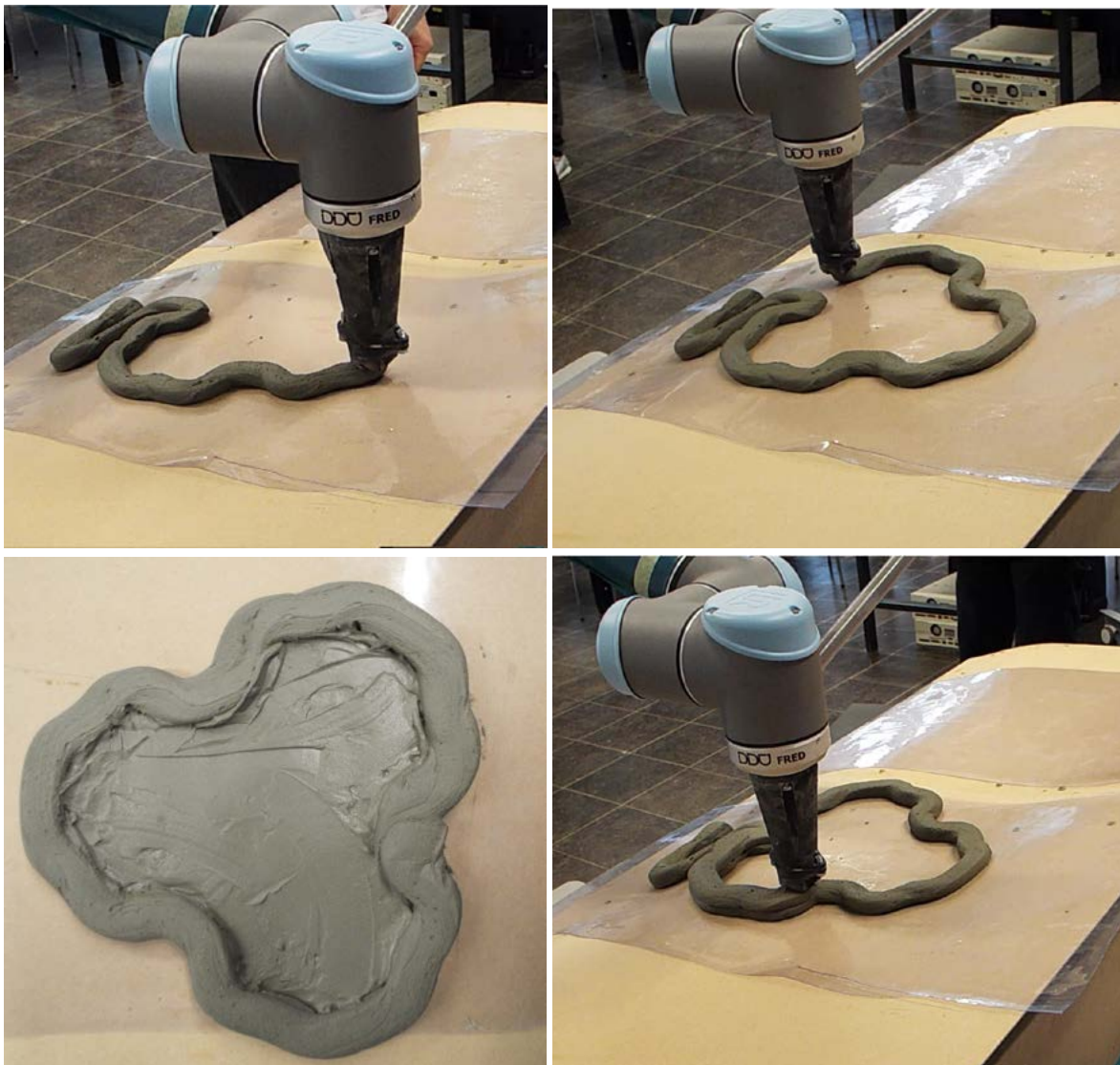
Figure 98 - Printing of stacked filaments and casting source: Author
