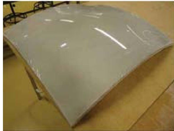
Figure 18 [top left] Fabric casting principles: Membrane is stretched across a pre-defined border into which concrete is cast source: Vergaeg, 2010
