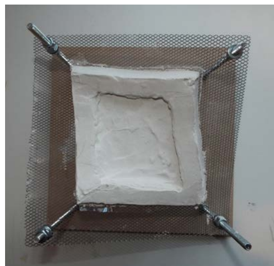
Figure 56 - initial prototype: extruded edges with cast cement source: author
