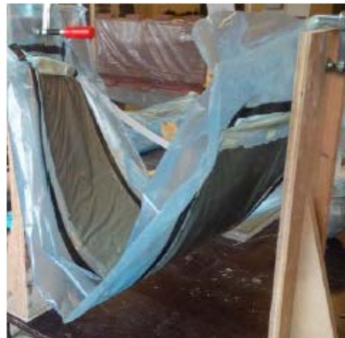
Figure 24 Developable concrete strip - Horizontal element transformed into arch source: F.Hubeijen, 2015
