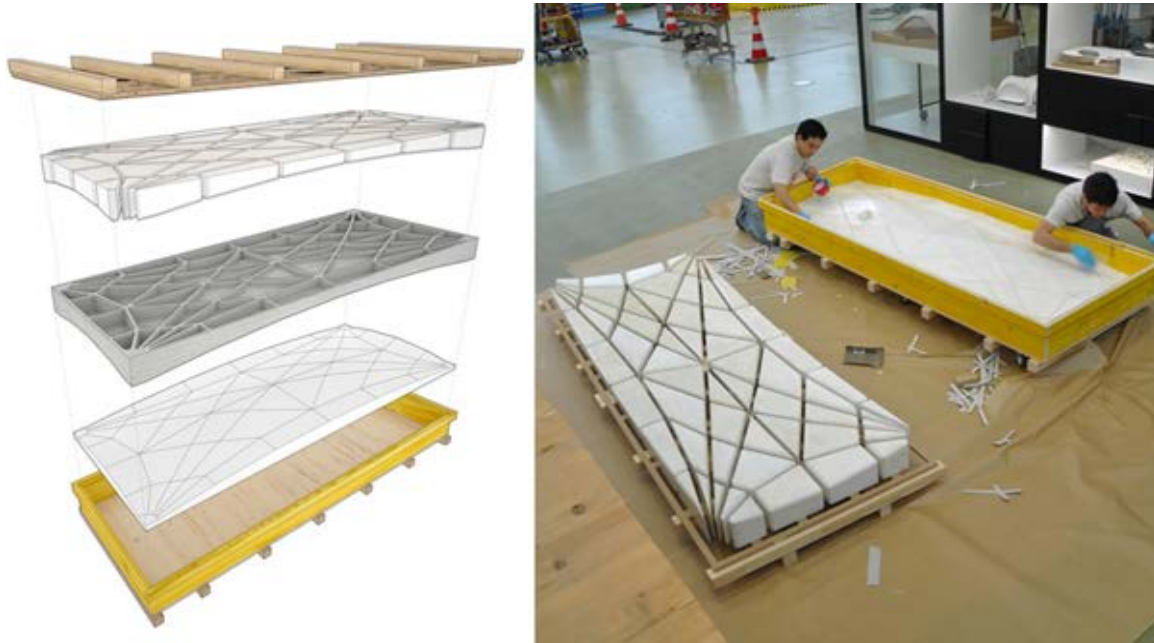
Figure 33: Use of multiple EPS Moulds to create rib-stiffened funicular floor system. The result is a neat and accurate geometry, however, is the manufacturing process efficient? source: ETH Block Research Group
