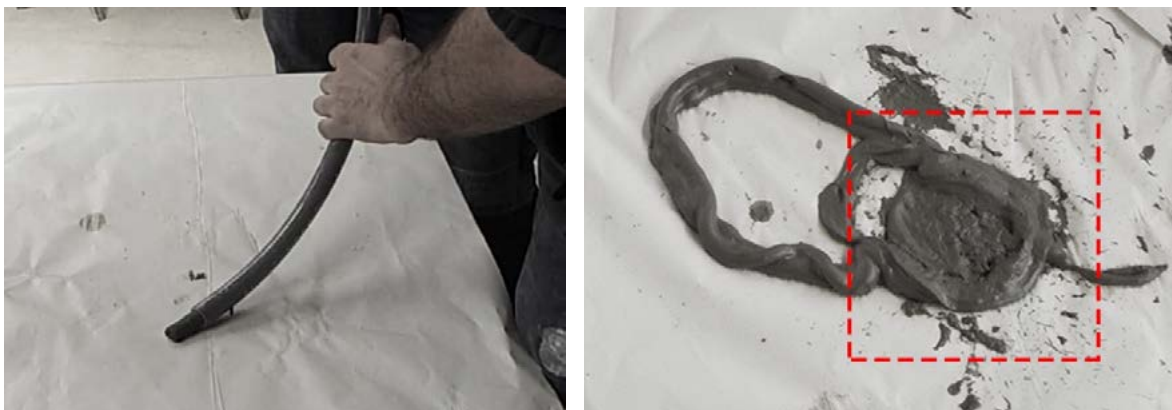
Figure 93 - Initial testing using pressure drive for material. [left] material too stiff and clogged in feed pipe. [right] material too fluid and prone to splatter source: Author
