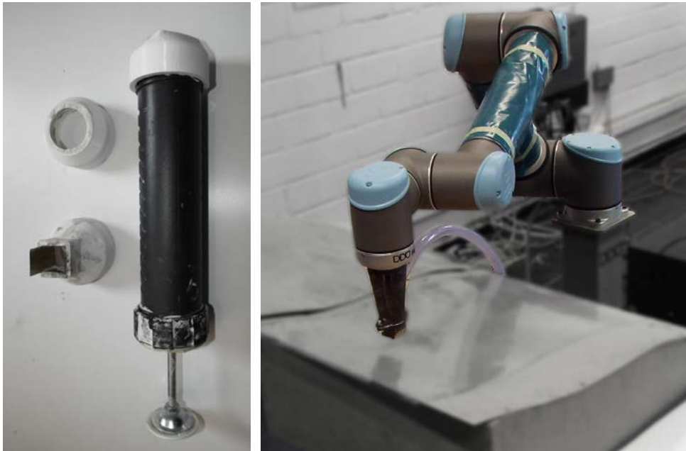
Figure 85 - evolution of mechanically-driven to pressure driven material deposition source: Author
