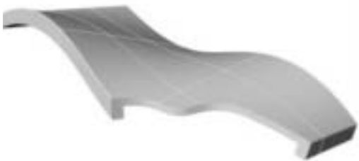
Figure 8 [top left]: Double curved concrete panels with additional geometric complexity: surface texture. source: author
