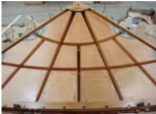
Figure 31: Wooden counter mould used into fabricate ribbed elements in Hilversum source: Herwijnen, 2005
