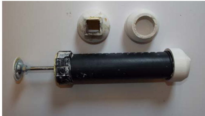
Figure 55 - end effector comprised from caulking gun source: author
