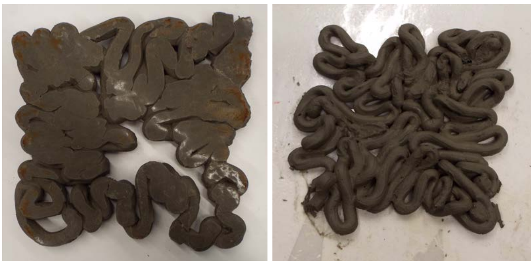
Figure 102 - Printing of fully-printed panel prototype source: Author
