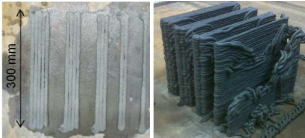
Figure 52- [left] Test example of extrudability tests in concrete. [right] buildability tests in concrete source: Buswell, 2010
