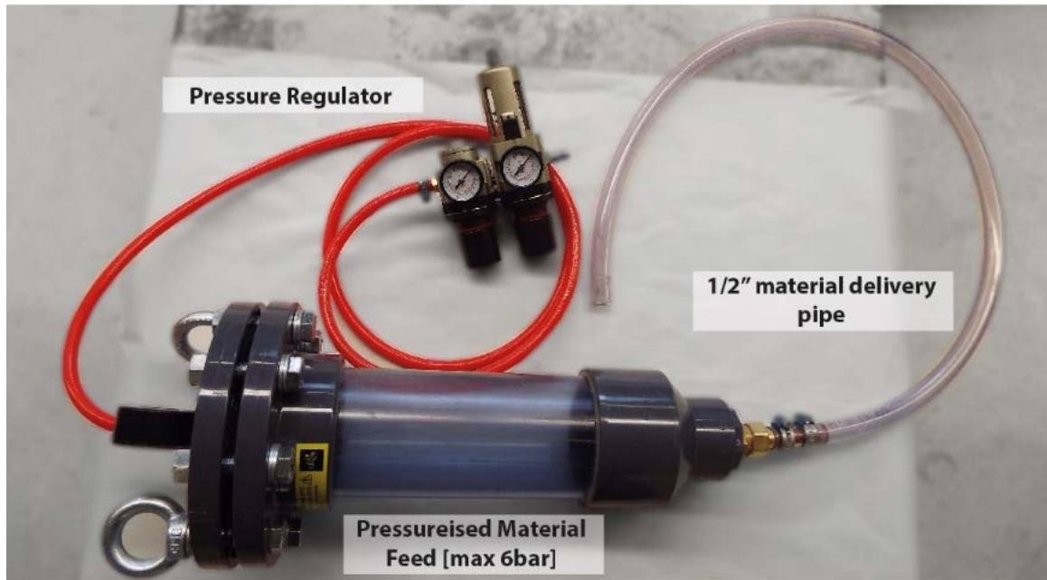
Figure 88 - Pressure-driven system setup source: Author
