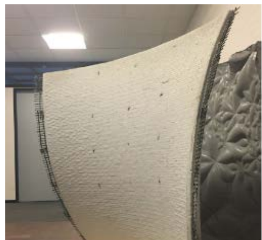
Figure 26: Hybrid manufacturing technique using CNC-Milling and Additive Manufacturing - Prototype Source: Silva, 2015
