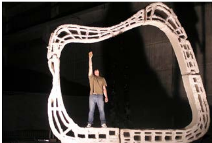
Figure 42 - D-Shape Printing Process in hypothetical building source: D-Shape.com
