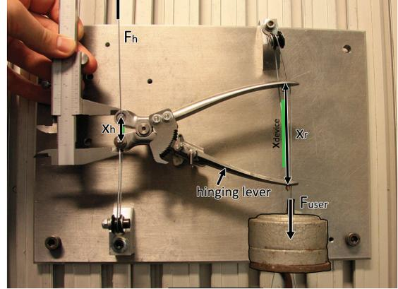
Figure 25: Experiment setup to evaluate the amplification function of the device in traditional and amplifier mode.
