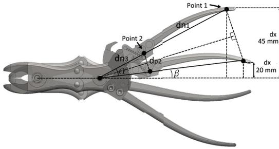
Figure 19: Dimensions and angles used for calculating necessary displacement of point 2 ( $d_{p2}$ )
