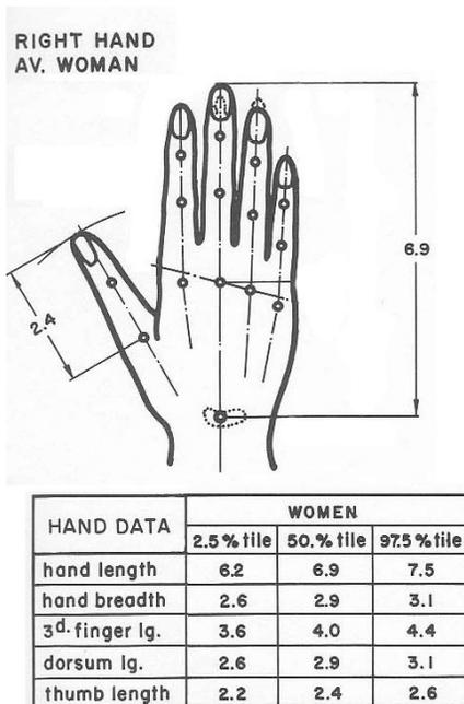
Figure A.32: Maximum hand span in inches. Adapted from [21] ]
