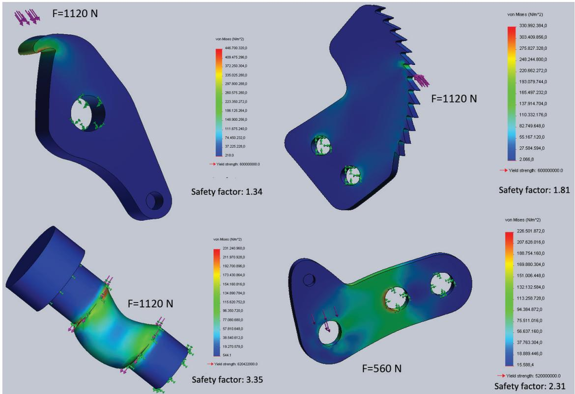
Figure 21: Solidworks Xpress stress results of critical parts, loaded with the calculated forces from Table 5 and in the directions shown in Figure 23.
