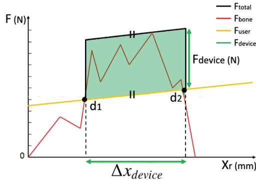
Figure 3: The force necessary to advance the rongeur beak through the bone,  $F_{bone}$  (simplified to  $F_{total}$ ), exceeds the users maximum gripping force,  $F_{user}$ , during the interval  $\Delta x_{device}$ . During this interval, assistance from the device is needed, either by amplifying the user gripping force or adding force.  $x_r$  is the instrument handle span, further illustrated in Fig. 4
