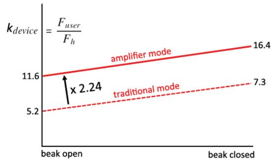
Figure 17: Amplification ratio of the device in traditional and amplifier mode, simplified to linear relation. In traditional mode, the device has the same amplification as the unchanged rongeur. In amplifier mode, this amplification is increased 2.2 times, as determined necessary (section 2.1.2. For meaning of symbols, see Fig. 16)
