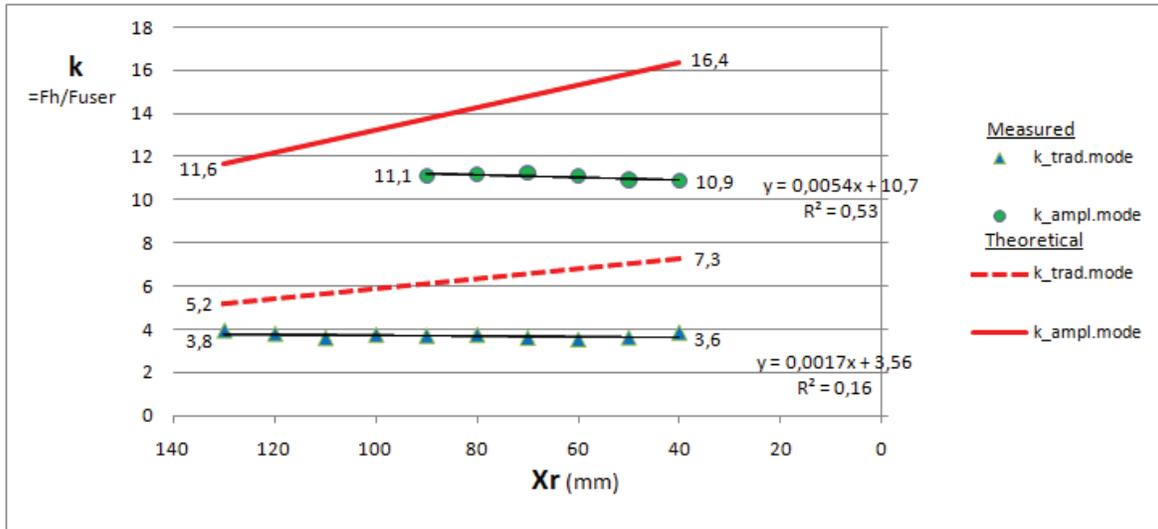
Figure 26: Theoretical and measured amplification factor  $k$  in traditional and amplification mode
