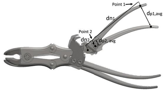
Figure 20: Dimensions and angles used for calculation of the average displacement of point 2 ( $d_{p2,avg}$ ) for the average closing distance ( $d_{p1,avg}$ )
