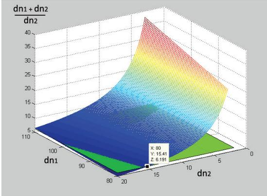
Figure 18: All combinations of  $dn_1$  and  $dn_2$  on the green patch create a wanted new amplification factor (11.6-16.4x). The highlighted point was selected based on the boundary conditions:  $dn_1 = 80$   $dn_2 = 15.4$
