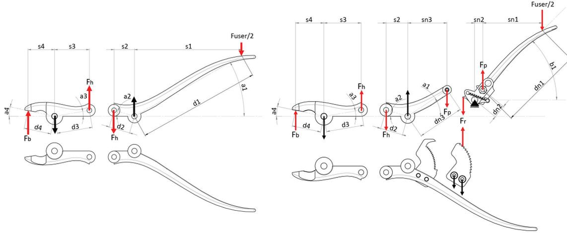
Figure 16: Static analysis of current rongeur (left) and device (right). The bottom half of the instruments is assumed fixed for calculation purposes. All forces in y-direction were considered and the values shown in Table 4. The triangle indicates a point that is assumed fixed because the pawl locks into the ratchet. The amplification ratios are defined as as input force  $F_i$  divided by  $F_h$ .
