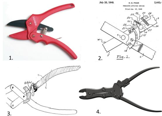
Figure 10: Inspiration for the final concept came from a ratchet pruner (1), and with the help of a patent [18], evolved (3) into the current design (4).
