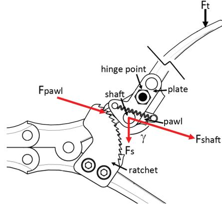
Figure 23: Load directions on critical parts
