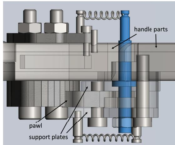
Figure 15: The connection shaft, shown in blue, has several extrusions to prevent handles from generating too much friction with one another, but still enable the support plates to be bolted firmly onto the handle.
