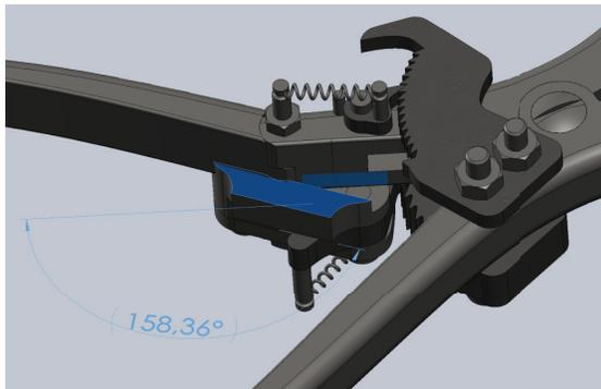
Figure 11: The handle blocker, shown in blue, prevents the active handle to make an angle over 180 degrees with the rest of the handle because it is blocked by the rest of the handle (light blue patch). This way, the device can still be used in normal mode without using the amplification.
