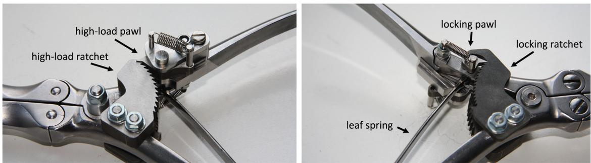
Figure 22: The prototype. The front contains the mechanical amplifier with the high-load pawl and ratchet. The back of the device contains the locking pawl and ratchet, which keep the beak section in its position when the handle is retracted.
