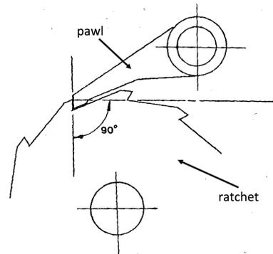
Figure 12: Ratchet design rule of thumb: A line perpendicular to the face of the ratchet-wheel tooth must pass between the center of the ratchet wheel and the center of the pawl pivot point to prevent the pawl pushing itself out. [19]
