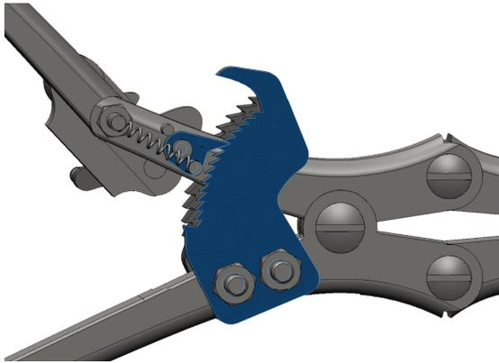
Figure 13: Back of the device showing ratchet and pawl that keep the beak section from opening when the device handle is retracted for another squeeze.
