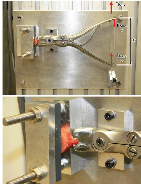
Figure 4: Setup imitating cutting of an osteophyte. A pull-bench pulls the rongeur handles closed and measured the necessary bone cutting force as a function of handle span, plotted in Fig. 5
