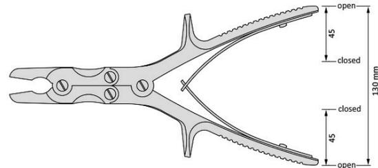
Figure H.46: Rongeur handle span in opened and closed state
