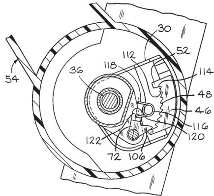
Figure 14: The idea of the design of the bi-stable system and especially the part flipping the pawl in its end states, came from the armrest in passenger cars. This figure shows the patent from Bart [20] for such an armrest which was used as inspiration.
