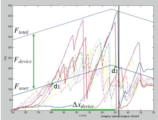
Figure 5: Plot of some of the bone cutting runs (measured at the end of the rongeur handles). Simplified bone cutting force  $F_{total}$  and user gripping force  $F_{user}$  are shown, as well as  $\Delta x_{device}$ .
