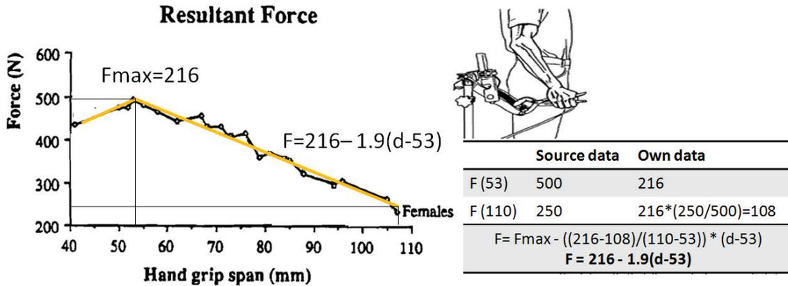
Figure A.31: Influence of hand span on gripping force for women. Existing data was used to derive the relationship between hand grip span and gripping force. Adapted from [ ]
