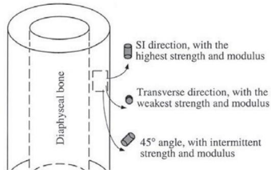
Figure D.40: Bone cutting direction. The bone cutting direction is one of the factors influencing the bone cutting force.[12]
