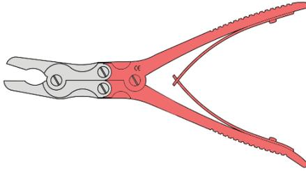
Figure 8: Handle section of rongeur shown in red. Because many problematic instruments are based on the same construction, the handle parts can be exchanged.
