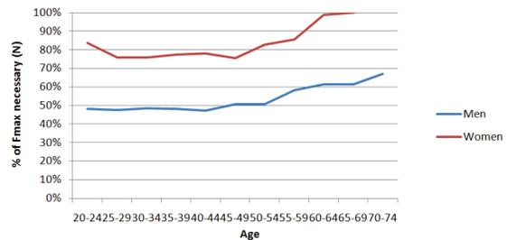
Figure E.43: Device enables weakest person to cut all tissues. This means that all users with more gripping force can now cut the hardest tissues without using their maximum gripping force
