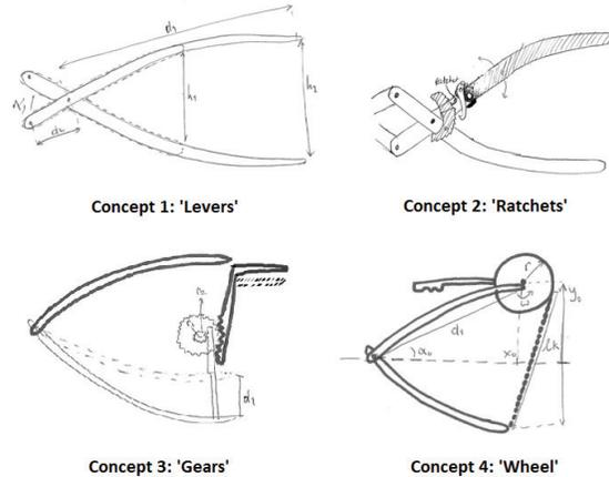
Figure 9: The four concepts. Concept 1: elongated handles. Concept 2: extra amplification enabled by retracting handle and a ratchet-pawl system. Concept 3: two gears on the same shaft amplify gripping force. Concept 4: a wheel and chain amplify user gripping force. For further explanation of the concepts and a technical analysis, see Appendix I
