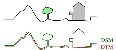
Figure 1.1: Top: a terrain with a mountain, a tree, and a building. Bottom: its DSM and DTM.
