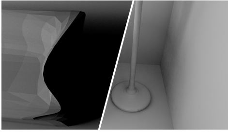
Figure 9: Comparison between global illumination using photon mapping (right) and only direct lighting (left), both using ReSTIR DI. 500 frame accumulation.
