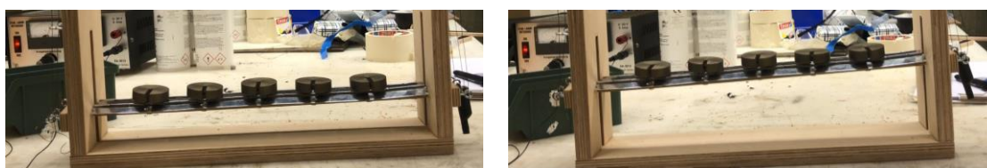
Figure 127, Mock-up 1, frame test without glass
