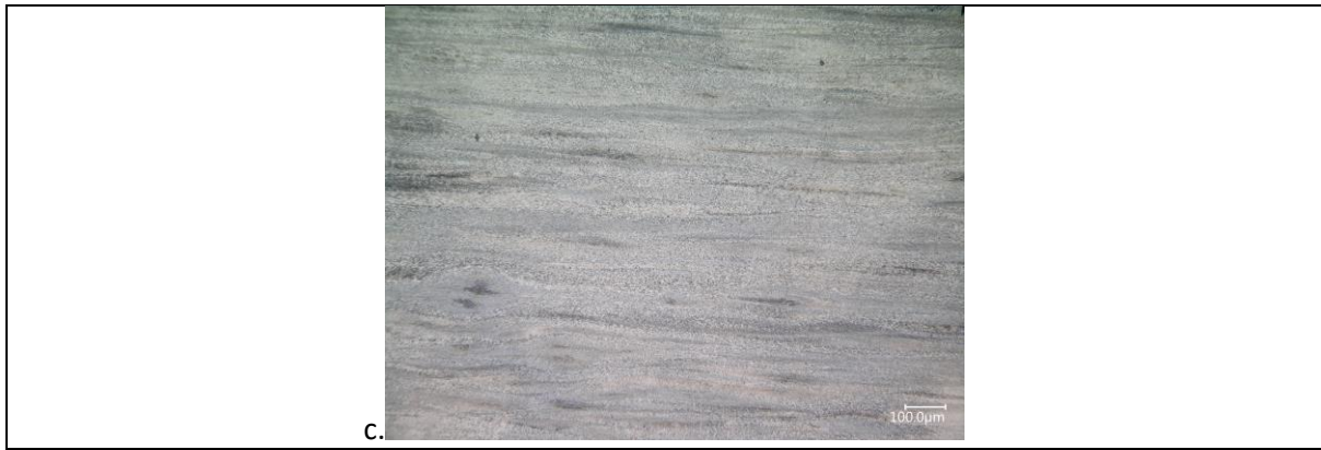
Figure 66 Optical micrographs of etched as rolled FeNiCrCoAl high entropy alloy after 800°C heat treatment for (a) 16 hrs (b) 24 hrs (c) 48 hrs
