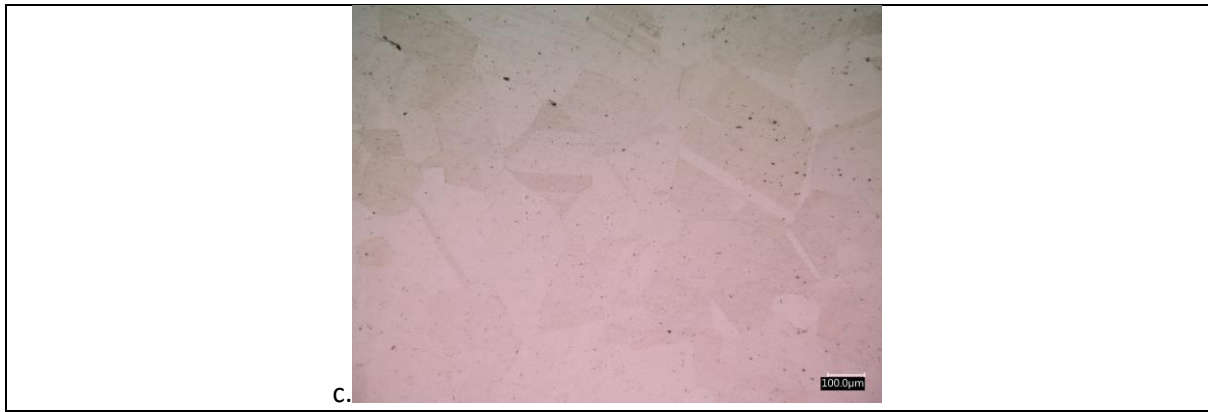
Figure 58 Optical micrographs of etched as rolled FeNiCrCo high entropy alloy after 1100°C heat treatment for (a) 16 hrs (b) 24 hrs (c) 48 hrs
