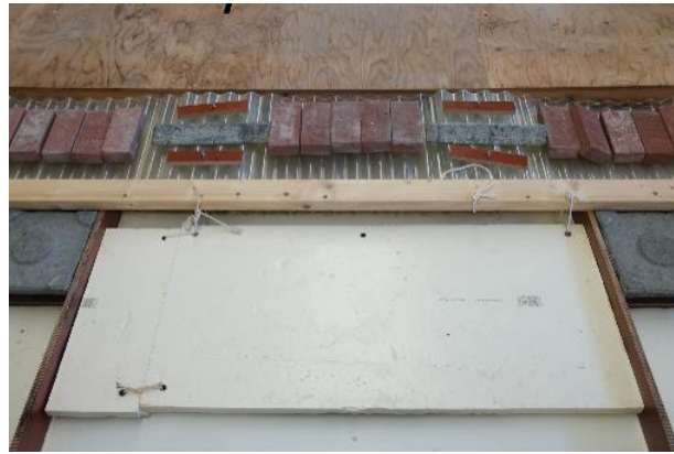
Figure A.2: Honeycomb and foam board to damp disturbances issued from the inlet section.
