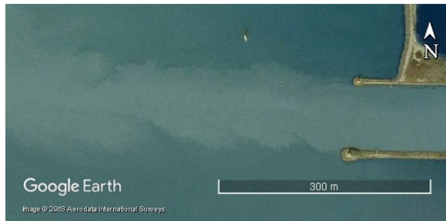
Figure 2.15: Shallow turbulent jet: the outflow of the river IJssel, The Netherlands (source: Google Earth 2018).
