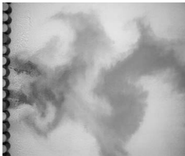
Figure 2.19: Dye visualisation of grid turbulence (Uijttewaal and Jirka, 2003).
