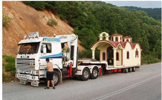
fig.15: transport of a pre-fabricated byzantine-style chapel by the firm Markaris on a flat bed truck, Greece. Markaris Company Website.
