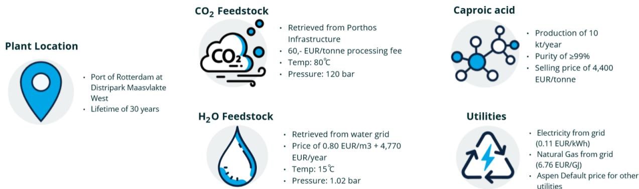
**Figure 3.2:** Schematic summary of the identified plant location, feedstock sources, product properties and utilities.
