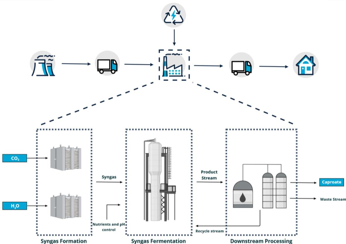
**Figure 3.1:** Schematic Overview of the scope of the process design and performance assessment. The scope is limited to a gate-to-gate design, excluding feedstock production and transportation, (renewable) electricity production and product distribution. Within the scope of this research are; pre-treatment of the feedstream, syngas formation via electroreduction of  $\text{CO}_2$  and  $\text{H}_2\text{O}$ , *n*-caproate production via syngas fermentation and downstream processing.
