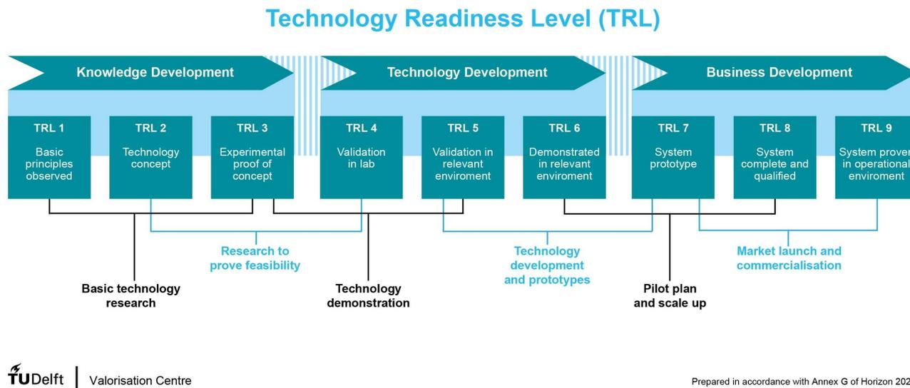
**Figure 1.2:** Overview of the Technology Readiness Level scale. This scale is used by the European Union to indicate the position of a technology. Retrieved from: *E-refinery 2022*.
