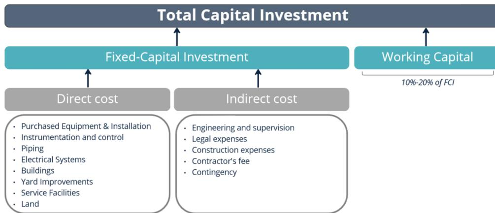
**Figure 4.8:** Schematic overview of the bottom-up approach. The total capital investment is calculated by retrieving the direct and indirect costs from Aspen Process Economic Analyzer. Based on these costs, the fixed capital investment (FCI) is retrieved. The working capital investment is 10%-20% of the FCI. Combined they form the total capital investment.
