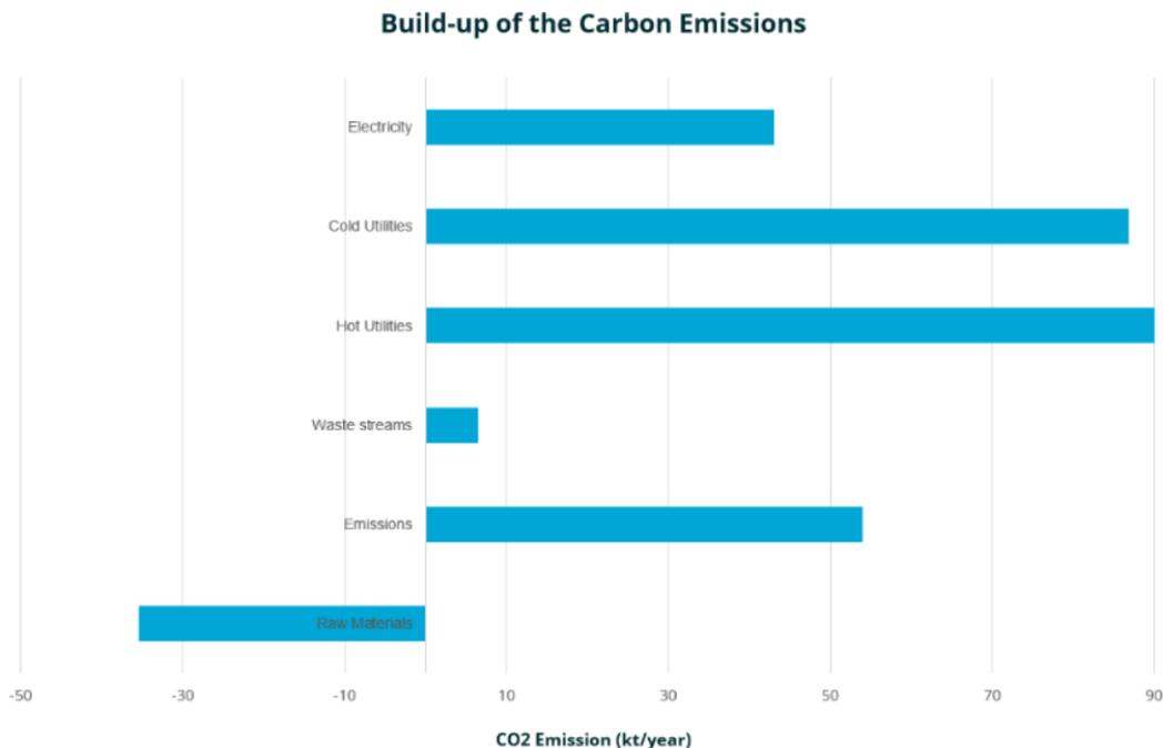
**Figure 4.10:** Overview of the contribution of the raw materials, waste streams, emissions and utilities to the total annual carbon emissions of the indirect route. The raw material input shows a negative carbon emissions, since it is dominated by the Porthos stream. Utilizing this CO<sub>2</sub> stream has a carbon emission factor of  $-1 \text{ kgCO}_2, \text{ emitted/kgCO}_2$ .
