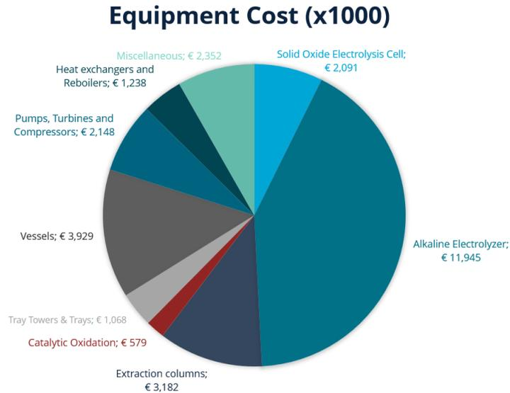
**Figure 4.9:** Component breakdown of the equipment cost. Cost are retrieved from the Aspen Process Economic Analyzer or manually calculated as explained previously. The costs are shown in x €1000. The total equipment cost are € 28.53 million and dominated by the alkaline electrolyzer of €11.95 million.
