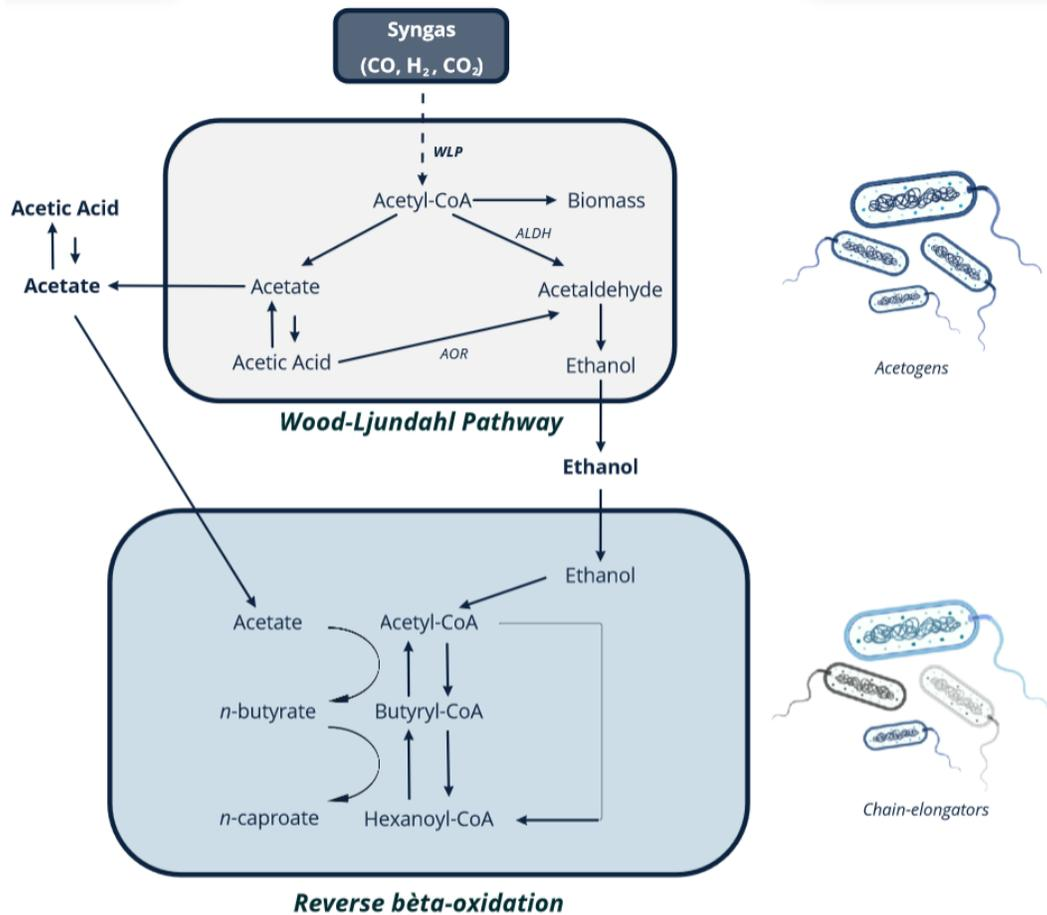
**Figure 3.10:** Schematic overview of the metabolic pathways used for: 1) syngas conversion into acetate and ethanol and 2) acetate and ethanol fermentation into medium-chain fatty acids (*n*-butyrate and *n*-caproate). Conversion 1 occurs via the Wood-Ljungdahl Pathway and 2 via reverse  $\beta$ -oxidation cycle (Fernández-Blanco et al. 2022).
