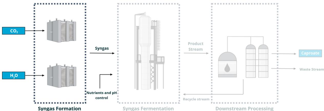
**Figure 3.3:** Schematic overview of the focus areas of section 3.2. These focus areas are the  $\text{CO}_2$  electrolysis, the  $\text{H}_2\text{O}$  electrolysis and the pre-treatment of the Porthos stream.
