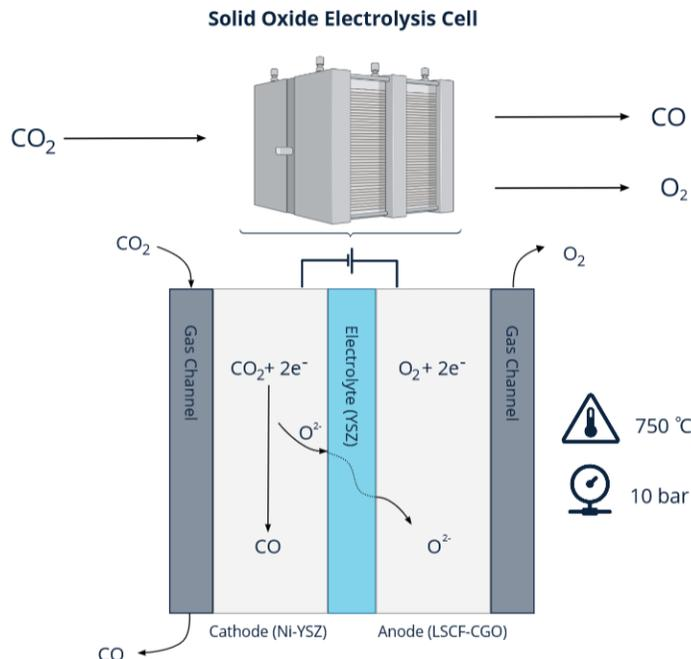
**Figure 3.5:** Schematic overview of the working principle of a solid oxide electrolyzer cell (SOEC). At the cathode  $\text{CO}_2$  is converted into CO. At the anode an oxygen atom reacts to form oxygen ( $\text{O}_2$ ).
