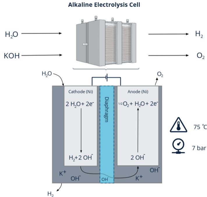
**Figure 3.8:** Schematic overview of the working principle of an alkaline electrolyzer. At the cathode  $H_2O$  is converted into  $H_2$ . At the anode  $OH^-$  react to  $O_2$  and water. 35 wt% aqueous potassium hydroxide (KOH) is used as liquid electrolyte.
