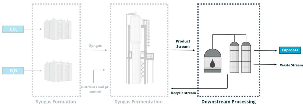
**Figure 3.11:** Schematic overview of the focus areas of section 3.4. These focus areas are the pH adjustment of the fermentation broth and reaching a *n*-caproate concentration of 99% in the product stream.
