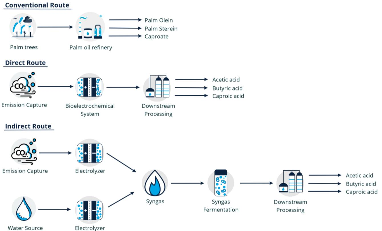
**Figure 1.1:** Schematic overview of the three *n*-caproate production routes. The conventional route uses palm or coconut trees as a feedstock. The direct and indirect route use CO<sub>2</sub>. In the direct route CO<sub>2</sub> is directly converted by microbial electrosynthesis. The indirect route produces syngas as intermediate. Based on Mba et al. 2015 and Wood et al. 2021
