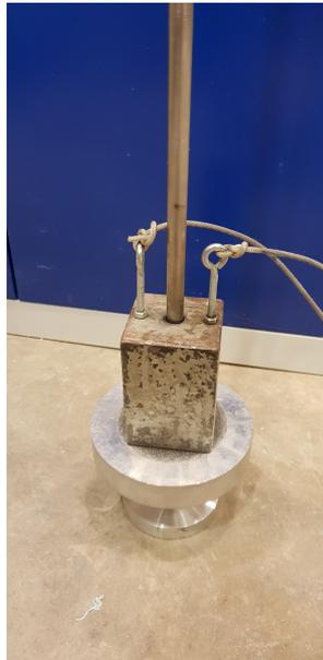
Figure 3.1: The hammer used for compaction; base plate diameter: 15.1 cm
