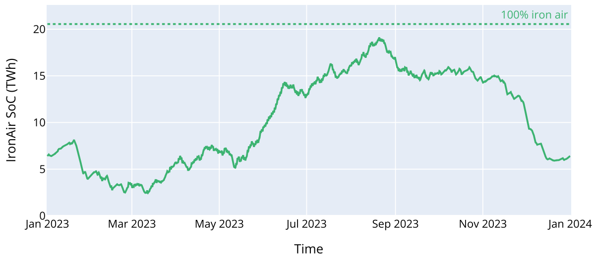
Figure C.26: State of charge of batteries for MDES-only scenario with 2040 demand
