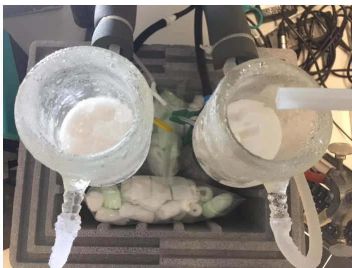
Figure 8. Sampling of ice (Left) and mirabilite (Right) during EFC process
