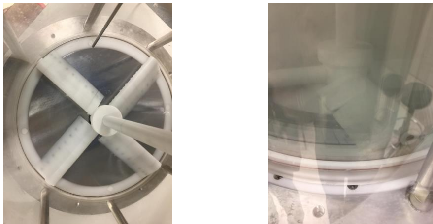
Figure 5. Top view of the stirrer with plastic-coating (Left) and ice scaling with uplifted blade (Right).
