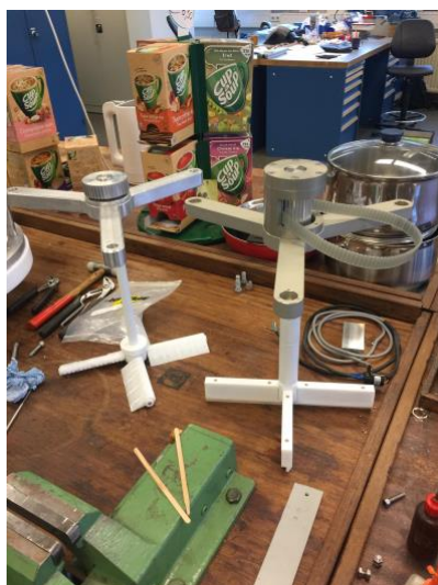
Figure 6. Inclined-blade stirrer (Left) and Vertical-blade stirrer (Right) sat on a table .
