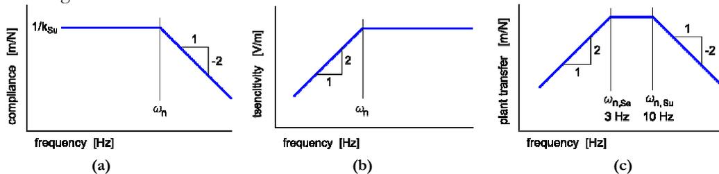
Figure 3-8 (a) The table compliance, (b) The sensor sensitivity and (c) The total plant transfer
