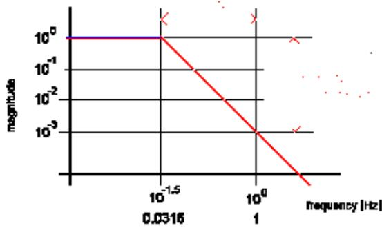
Figure 3 The natural frequency of linear springs needed for a 60 dB vibration attenuation at 1 Hz
