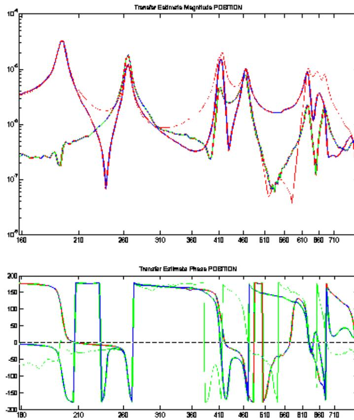
Figure 3-17 Bode diagram of three different sensor locations (bb,II), (m,II) and (ff,II)
