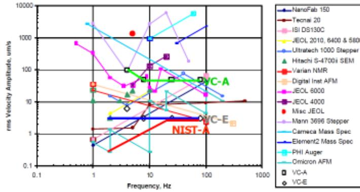
Figure 2-2 Specified maximum vibration levels for several high end systems
