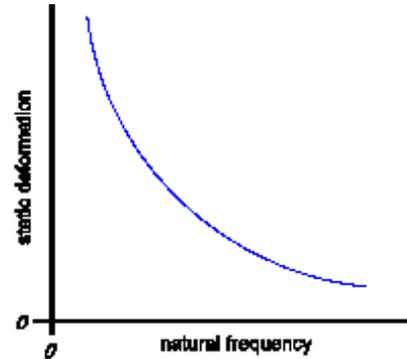
Figure (XXX) The inherent relation between natural frequency and static deflection for linear springs
