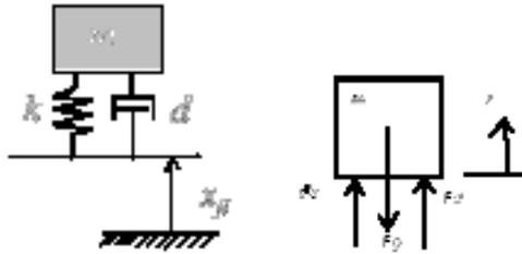
with  $F$  the force excited on the spring in Newton, and  $\delta$  the deflection of the spring in meter,  $\delta'$  the velocity of the deflection of the spring in Newton-seconds per meter.
