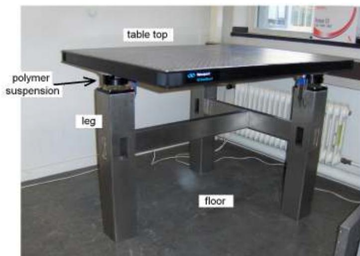
Figure 2-6 table with passive suspension
