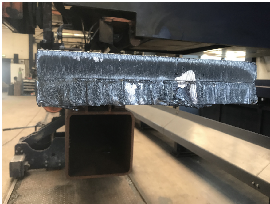
Figure 5-9: Cut with gouges due to air between two metal pieces
