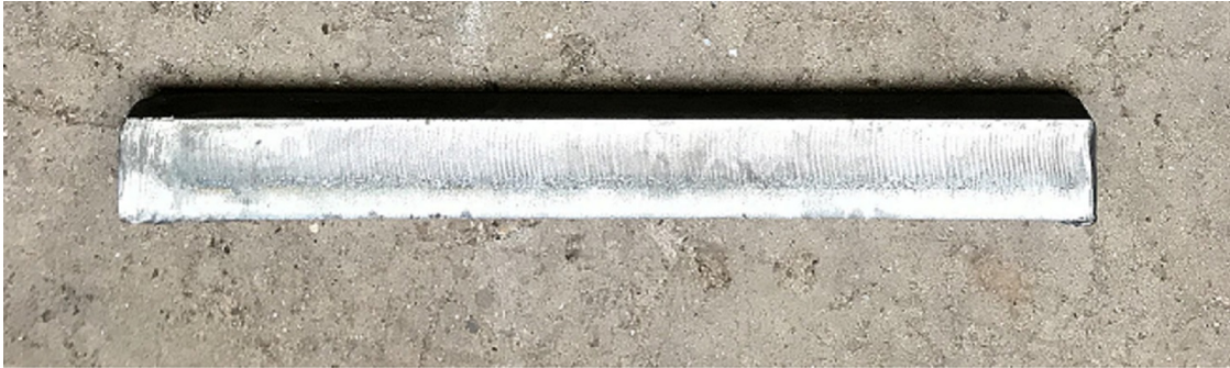
Figure 5-2: The cut having smooth plate surface with clean sharp edges free from slag
