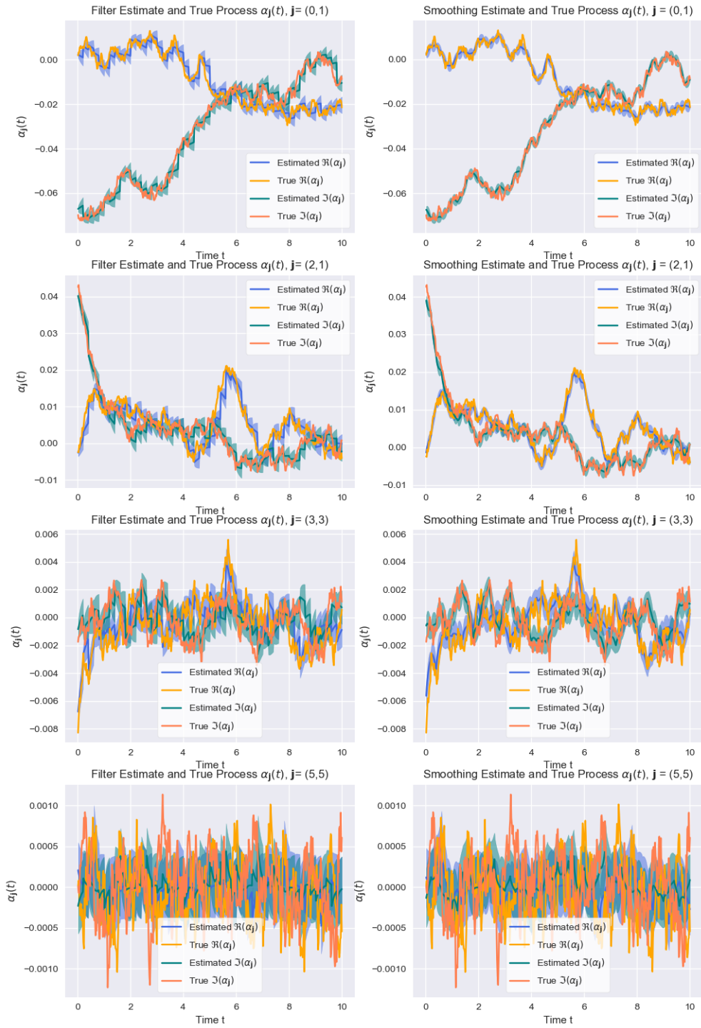
Figure 3.2.: Filtering and smoothing paths for differing spectral processes \alpha_j(t) . Different colors represent the true and estimated process for the real and imaginary part respectively. The shaded areas represent the mean estimate \pm the estimated standard deviation m(t) \pm \sqrt{K(t)} .
