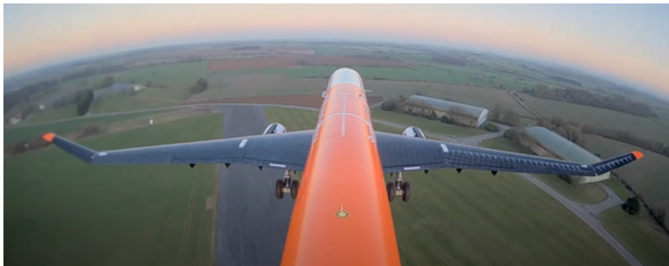
Figure 2.6: AlbatrossONE folding wingtips in GLA position, screenshot retrieved from [53].
