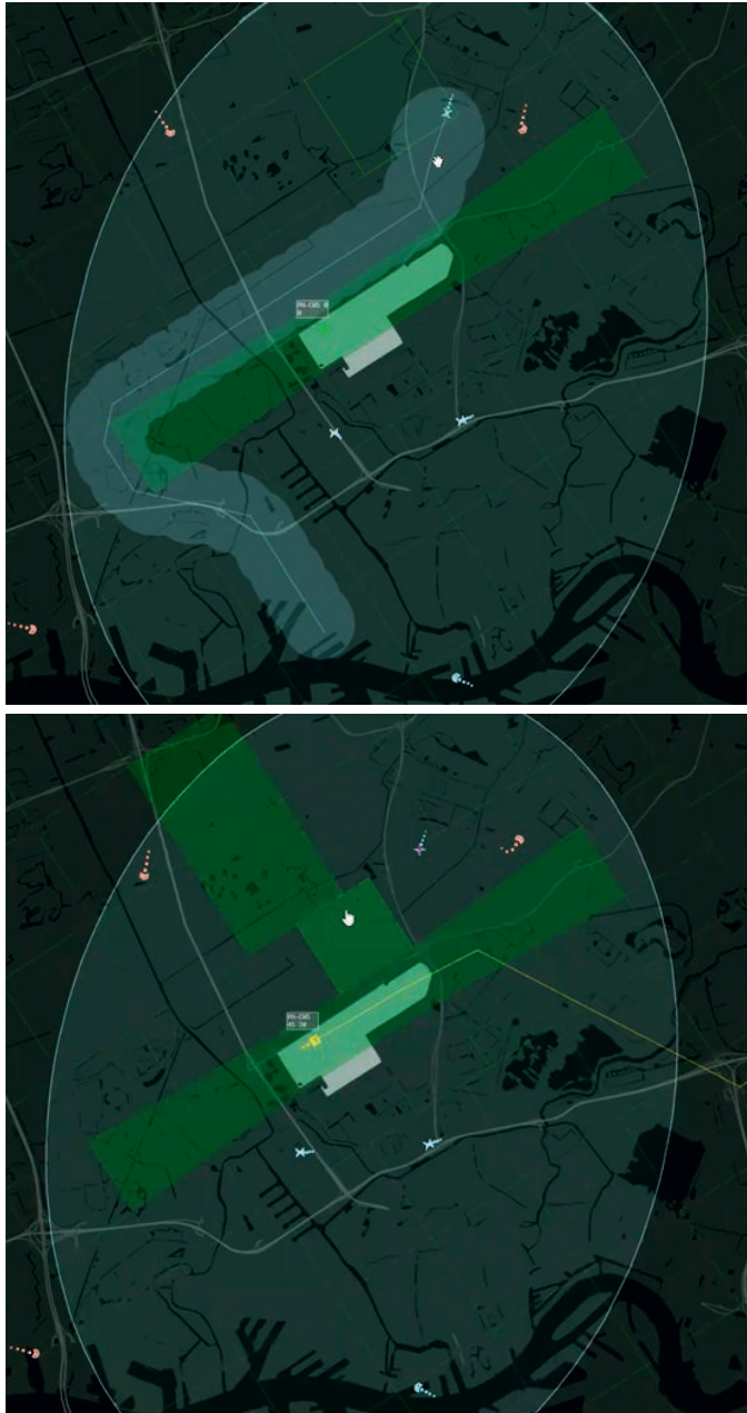
Figure 3.16: Utilization of geofences to force UAS loitering, rather than rerouting. The image above shows a UAS reroute due to short-term geofence restrictions. The image below shows how the UAS is forced to loiter by activating additional geofences.
