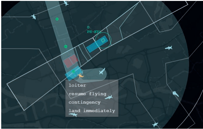
Figure 5.16: Use of UAS-specific commands to manage conflicts in the active control strategy.
