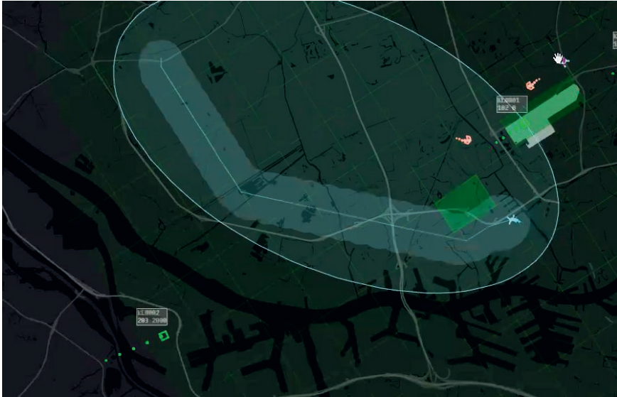
Figure 3.15: Geofence activated not to protect an area from UAS operations but to vector the selected UAS behind the landing crewed aircraft.
