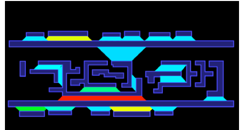
Figure 2.1: An image of a chip from IBM with the areas susceptible to shorts colored. Image is taken from [8]
