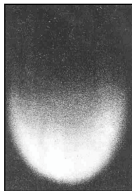
Figure 4.1: Bowl-like appearance of a falling group of spheres in air by (Slack, 1963)
