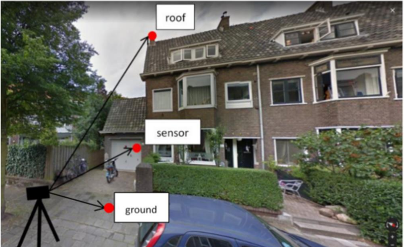
Figure B -0.2 Example of how the geodetic networks would have been established.
