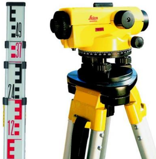
Figure 6.3 Instrument (level) and level staff( Source: http://www.surveyingequipment.com/product/leica-jogger-32-automatic-level-package/ )
