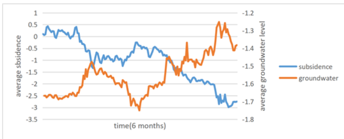
Figure 3.6 Correlation between subsidence data and water level data.
