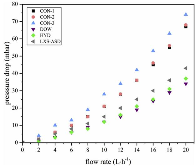
Fig. 6. Feed channel pressure drop (mbar) as a function of feed water flow (L·h<sup>-1</sup>) in MFSs for six different feed spacers: CON-1, CON-2, CON-3, DOW, HYD and LXS-ASD.
