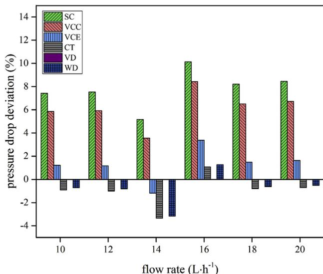
**Fig. 7.** Effect of different spacer porosity measurements on hydrodynamics for spacer HYD: The percentage differences in porosities can be translated into percentage deviation in pressure drop, with VD as reference method.
