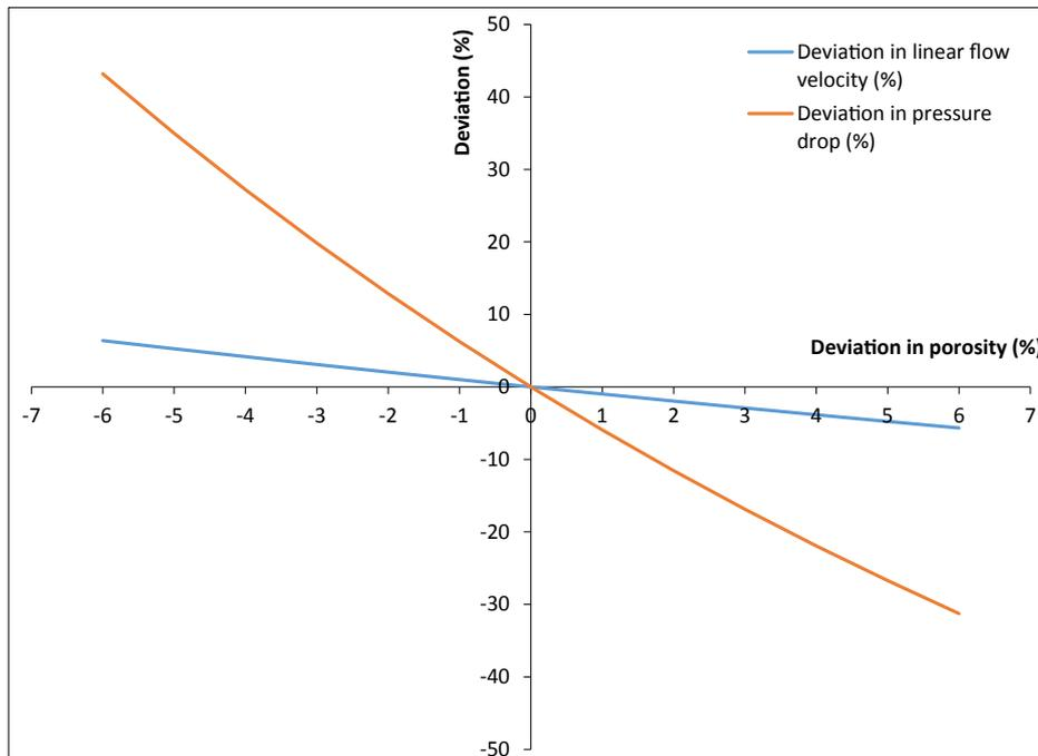
Fig. 5. Effect of feed channel porosity measurement deviation in percent (%) on linear flow velocity and pressure drop for a 34-mil thick standard spacer at a feed flow rate of 16 L·h<sup>-1</sup>.
