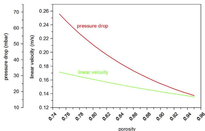
Fig. 1. Linear velocity and pressure drop calculations for a 34-mil (864  $\mu\text{m}$ ) thick standard spacer at a feed flow rate of  $16 \text{ L h}^{-1}$  and a feed channel porosity ranging from 0.75 to 0.95.
