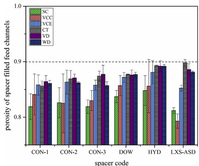
**Fig. 4.** Comparison of porosities of spacer filled feed channels in MFS for six feed spacers based on porosity methods: volumetric calculations: strand count (SC), cylindrical (VCC) and ellipsoidal (VCE), CT-scan (CT), volume displacement (VD) and weight and density (WD).
