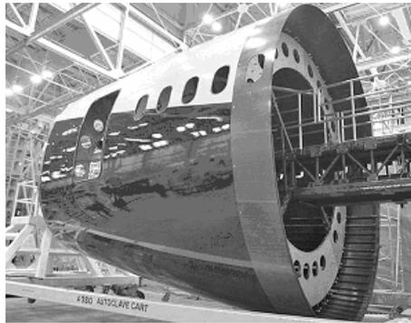
Figure 2.2: Impression of a CFRP Fuselage
