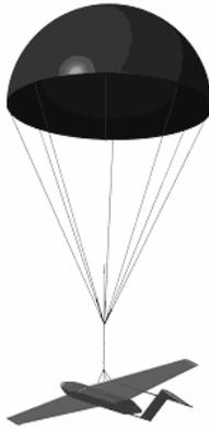
Figure 20.5: The SensAir UAV with deployed emergency parachute
