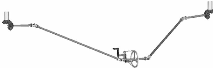
Figure 18.10: The Transmission system
