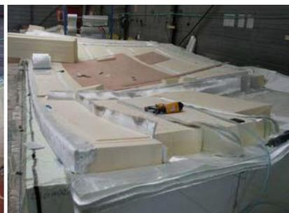
C. Laying out of polyurethane blocks on the cured exterior surface.
