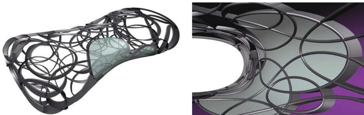
**Figure 85. Exemplary implementation of the scheme of tube-stiffened sheets in a structural design. In the zones with a transparent cladding the tubular structure continuous, whereas the sheets are interrupted.**
