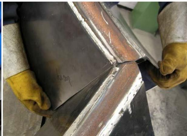
D. Positioning of two ribs of prototype 3.
