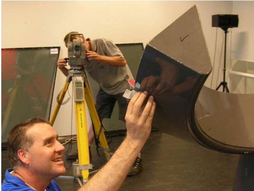
A. Measuring of the virtual intersection point of lines on adjacent surfaces.
