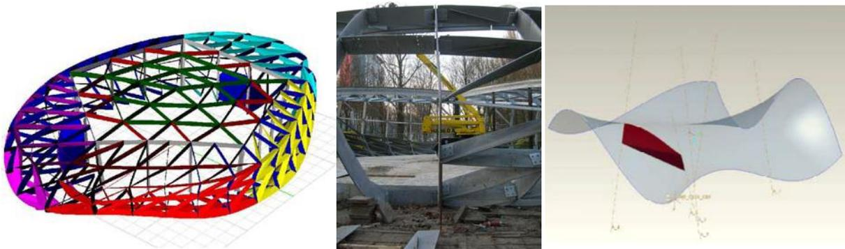
A. Digital model of the Web of North Holland: a steel sheet folded across its diagonal.
