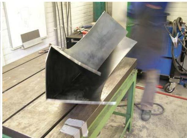
B. Three rib sides prior to positioning the tube inside it.
