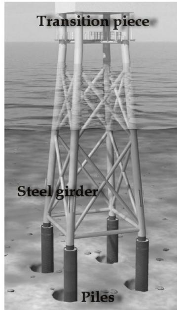
**Figure 2-2:** Example of a 4-legged jacket structure on piles (Cheng-Yu Ku and Lien-Kwei Chien, 2016).
