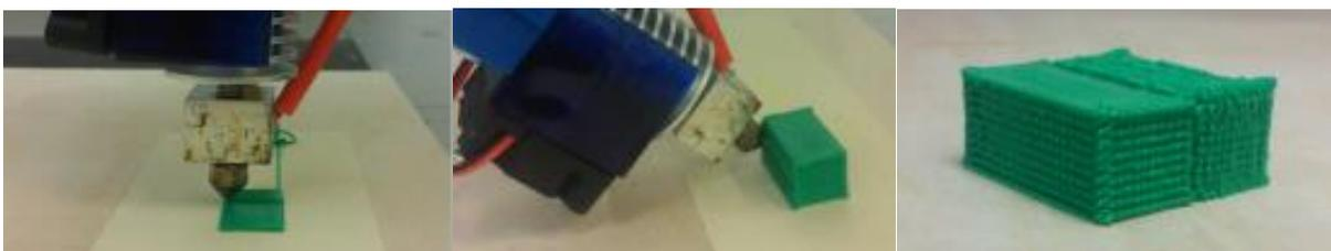
Figure 4 Blocks deposited from different angles. (I. Ishak, J. Fisher, & P. Larochelle, 2016)
