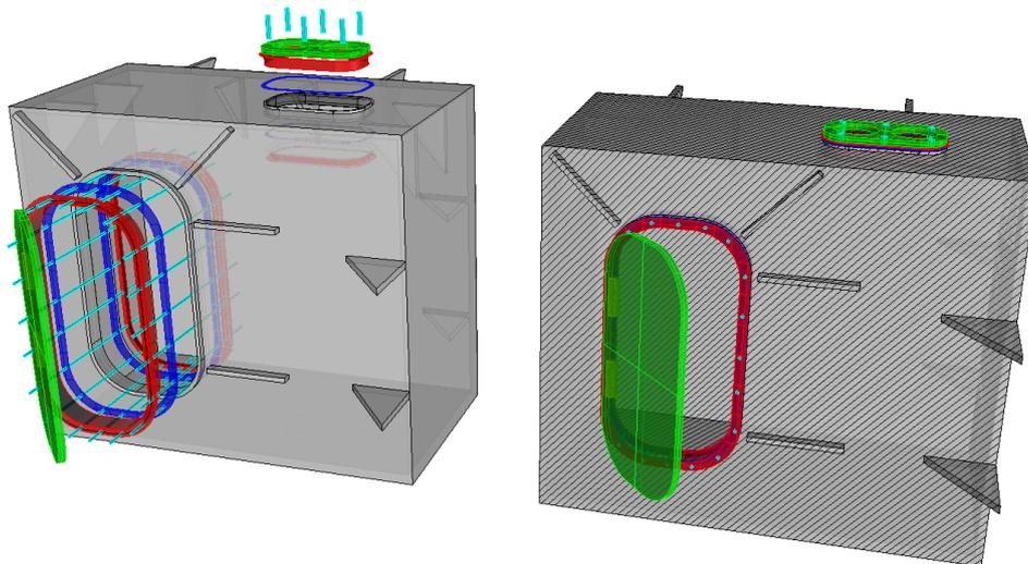
Figure 62 *Examples of a watertight door, a fitting and a series of lightening holes inside the double bottom.*
