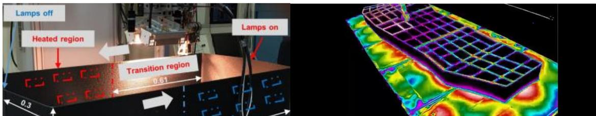
Figure 19 BAAM using infra-red to pre-heat previous layers. Thermwood using IR control. (BAAM / Thermwood)
