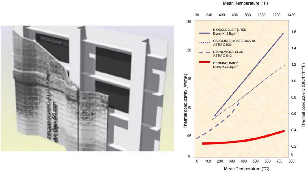
Figure 23 Various options for A60 class bulkheads as provided by PROMAGUARD
