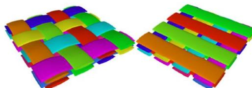
Figure 2 Woven (left) and cross-ply (right) laminate (T. Liu, Zhang, He, & Jia, 2017)
