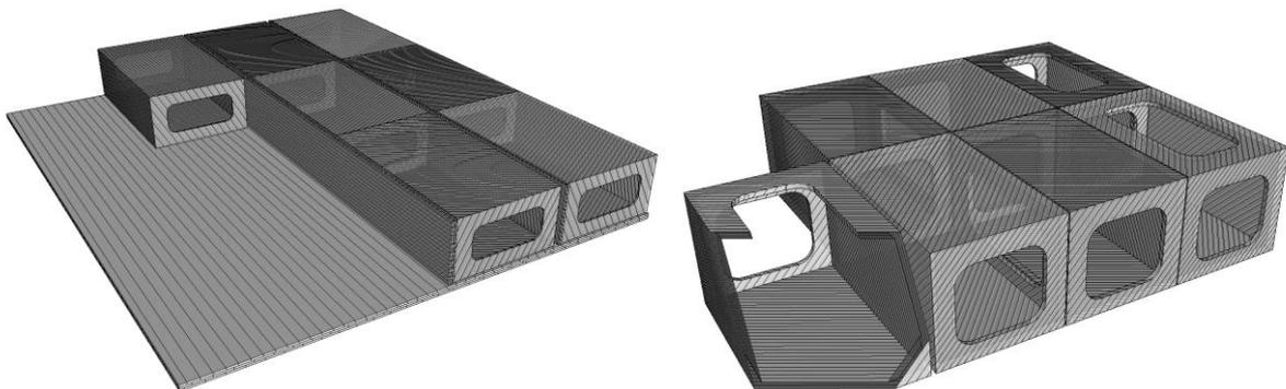
Figure 56 *Double bottom with in between girders and access holes*
