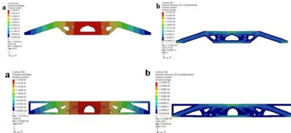
Figure 37 difference in optimization in and excluding a non-design space (Krishna et al., 2017)
