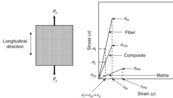
Figure 27 Stress – strain ratio matrix, fibre and composite (Mallick, 2007)
