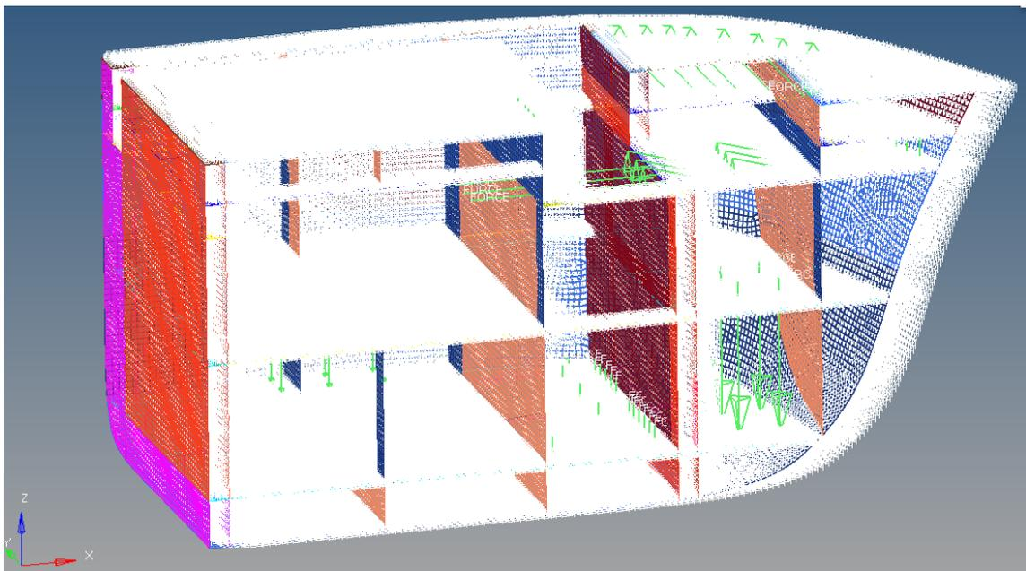
Figure 48 Laminate mesh including constraints, pressures (white arrows) and weight components (green)
