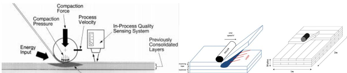
Figure 21 AFP technology and systems to control tape adhesion (Chinesta et al., 2014; Lamontia et al., 2003)
