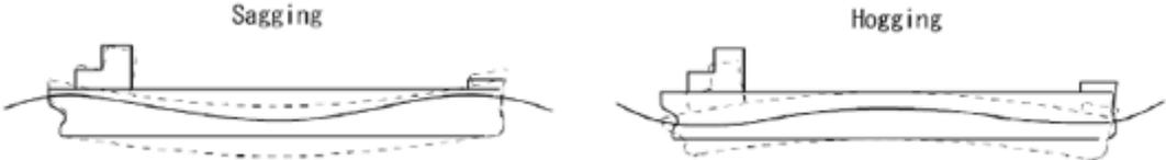
Figure Hogging and sagging (Buirma et al., 2017)
