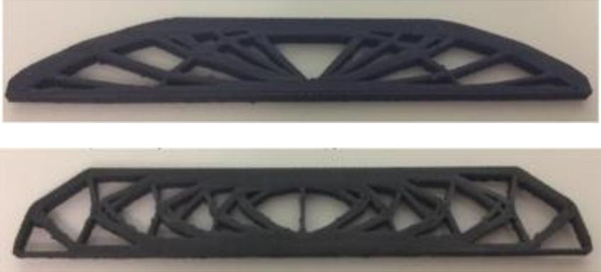
Figure 36 Horizontal and vertical AM strategy including orthotropic material behaviour in a 2D plane (Hoglund & Smith, 2015)
