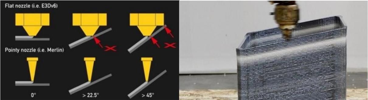
Figure14 Non-planar AM applied in small-scale AM-machines.(Rodriguez, 2016)
