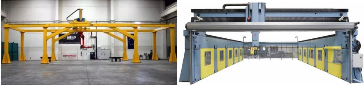
Figure 10 9 axis robot on a gantry and 6-axis metal-AM machine. (Kraken / 3D Hybrid Solutions - Multi-ax)
