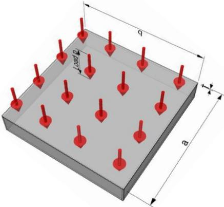
Figure 43 Deck plate element under pressure
