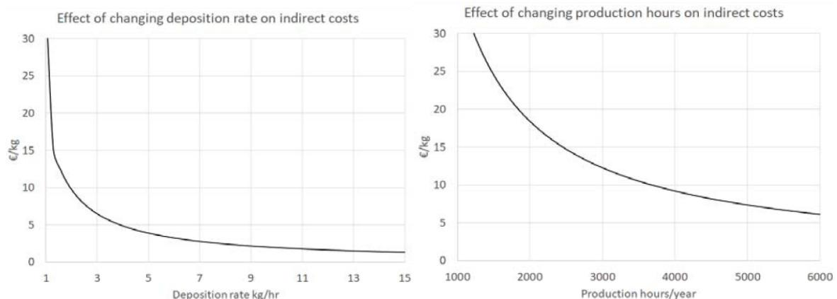
Figure 3 Deposition rate and production hours on EUR/kg (Buirma et al., 2017)
