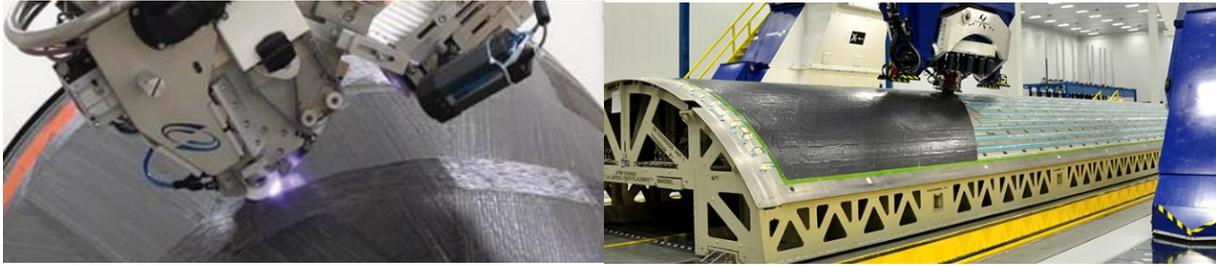
Figure 7 AFP of double curved smooth surfaces Coriolis/Electroimpact
