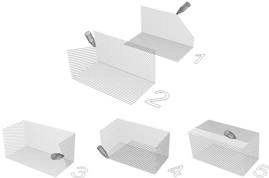
Figure 15 building up a hollow cube using multi-axis/non planar AM
