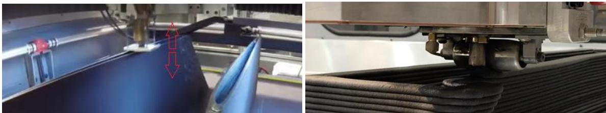
Figure 5 Tamper and roller to apply pressure deposition (BAAM / Thermwood)
