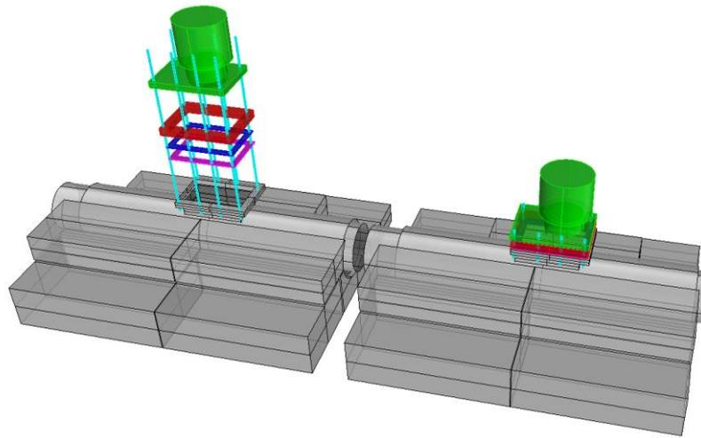
Figure 58 Option to assemble bow thruster unit in bow thruster tube
