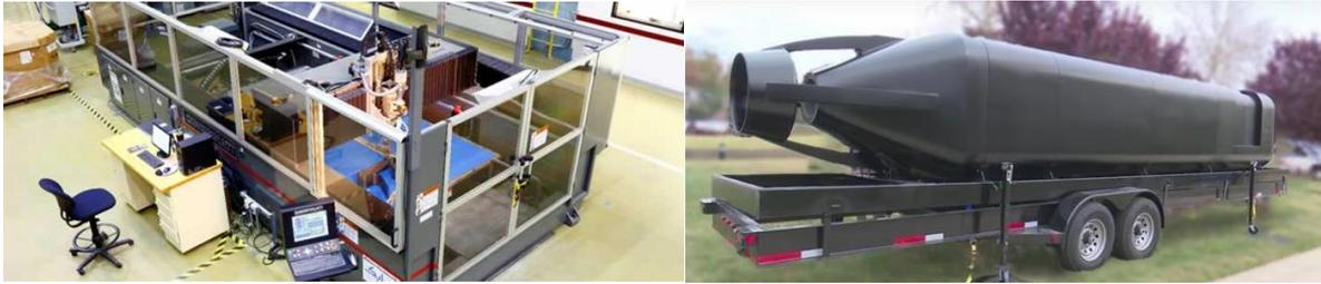
Figure 5 BAAM from ORNL and their largest 3D-printed asset at the moment
