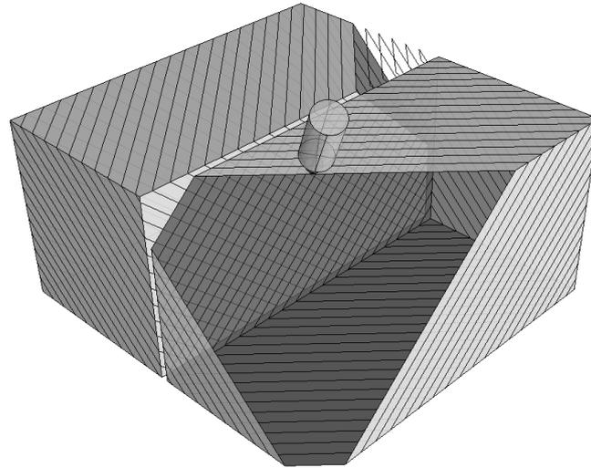
Figure 17 Multi-angle AM to produce cross-plyed divisions.
