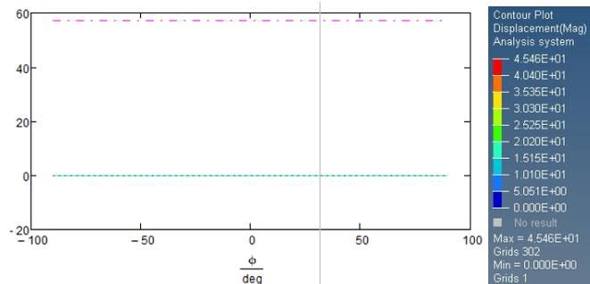
For a second thin plate with a force 100 times larger the deflection in MathCad showed 56 mm and the deflection in Hyperworks 45.4 mm. The difference is due to irregular loading in Hyperworks,
