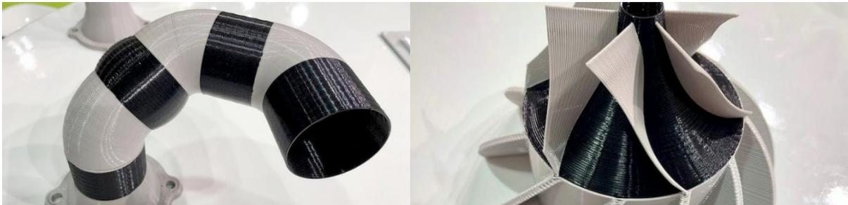
Figure 11 examples of FDM multi-axis additive manufacturing (V-shaper)
