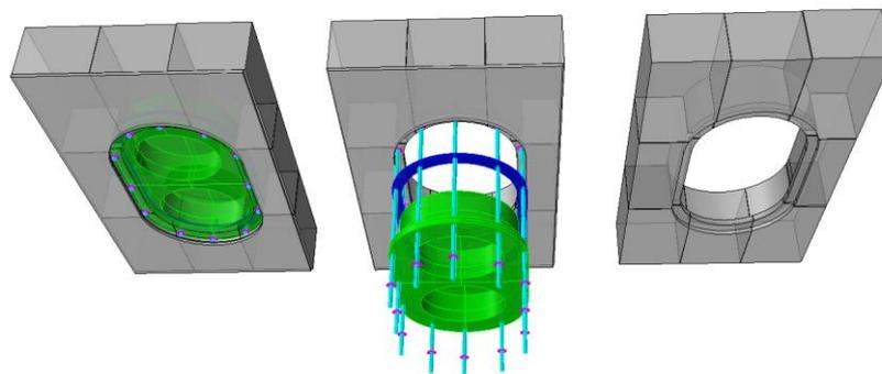
Figure 59 examples of the connection of the thruster unit in ship hull
