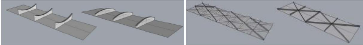
Figure 38 Options for plate stiffener configurations (Buirma et al., 2017)
