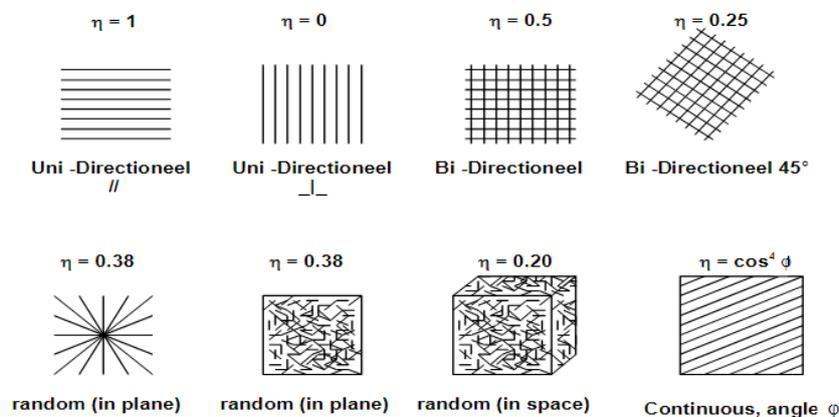
Figure 30 Effect of reinforcement resulting from orientation of the fibres. (lecture notes Kaminski 2018, TU-Delft)
