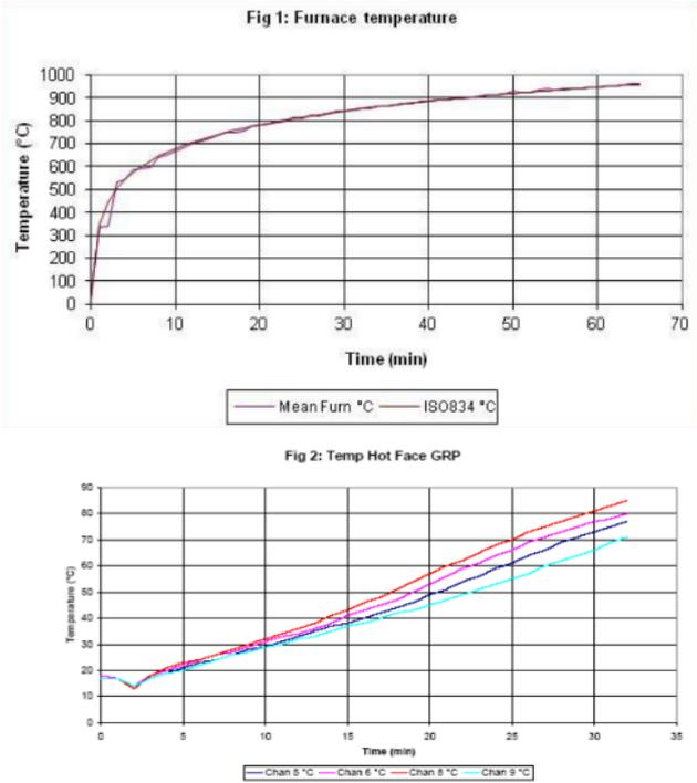
Figure 24 Furnace temperature created during a fire-test and corresponding temperature of hot side of FRP panel covered with 'Promaguard'.
