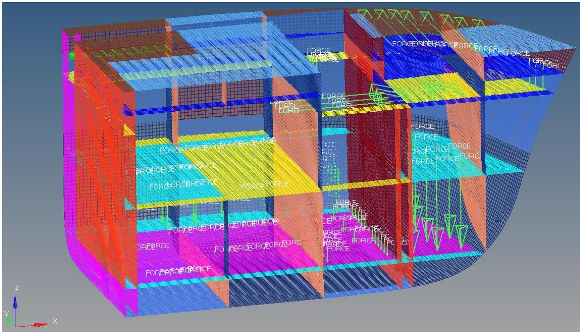
Figure 47 Laminate mesh including weight components (green)
