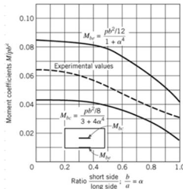
Figure 42 Accompanied graph to determine Moment coefficients based on ratio. (Boresi et al., 1985)
