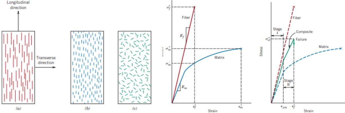
Figure 26 schematic representation of various fibre orientations and a schematic stress-strain curve for brittle and ductile material. (Clayton, 1987).
