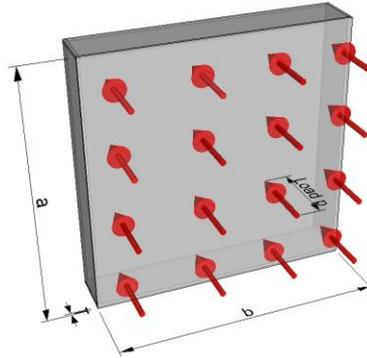
Figure 40 Outer plate element under pressure
