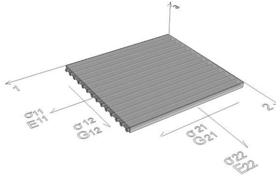
Figure 28 Transversely anisotropic laminate consisting out of one single ply.
