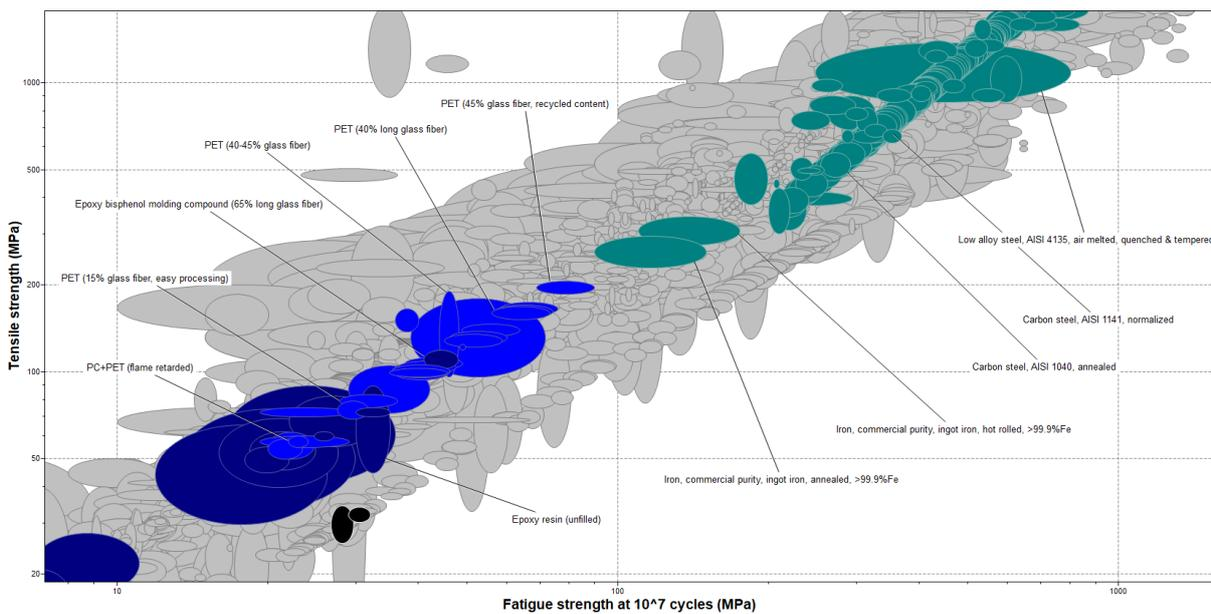
Figure 32 fatigue strength versus tensile strength of a wide range of PET (+PC) polymers (light-blue), metal alloys (green) and thermoset epoxies (blue) (CES.EduPack, 2018)
