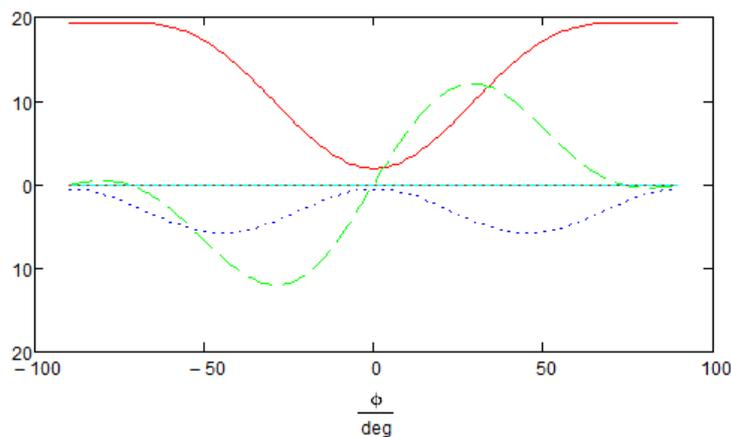
As can be seen from MathCad the deflection of the composite is approximately 19 mm when the fibres are oriented at 90 and -90 degrees and 2 mm when the fibres are oriented 0 degrees. In Hyperstruct these values are found to be 1.19 mm and 29.7 mm. the difference is due to the fact the MathCad code also takes into account the fibre E-transversal and matrix E-transversal and thus is more accurate:
