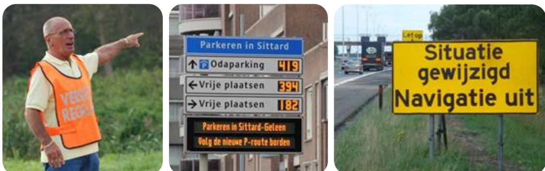
Figure 4: Basic route strategies - traffic controller (left), PRIS (middle) and advice to turn navigation device off (right)
