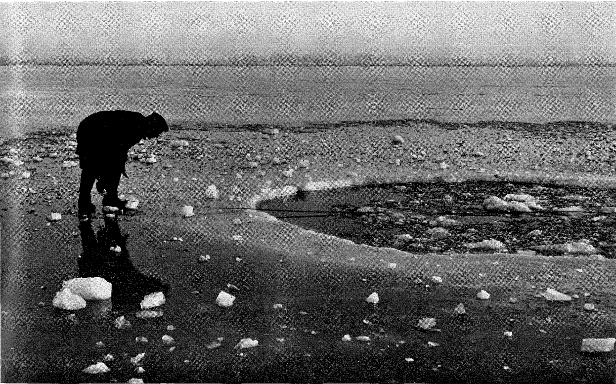
Measuring diameter of hole blown in ice.
