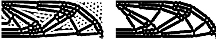
Figure 3.7: Maximum length scaling imposed morphological operations. Case 1: Maximum length scaling on both phases and Case 2: Scaling only on the solid phase. (Lazarov and Wang[68])
