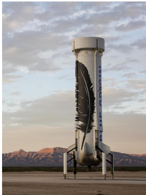
(a) New Shepard propulsion module. Image credit: Blue Origin
