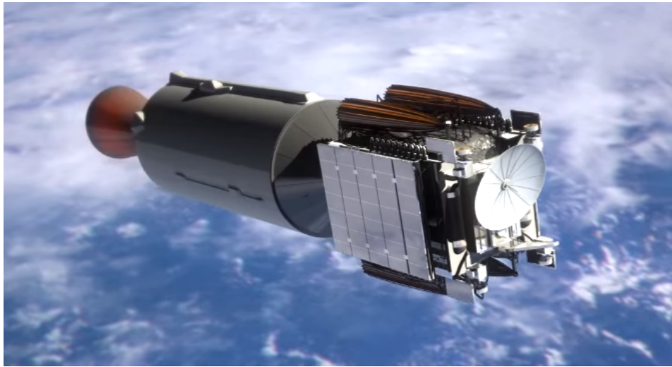
Figure 2.4: Rendition of the Falcon 9 second stage after engine cutoff still attached to the payload. Image credit: SpaceX
