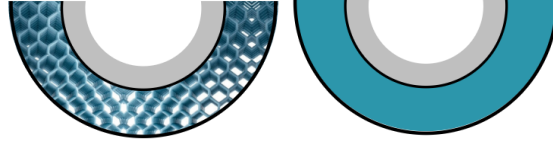
Figure 10: The actual implant design for the deformable cup (left) and the simplification (right). Grey displays the stiff titanium and blue the porous deformable part.
