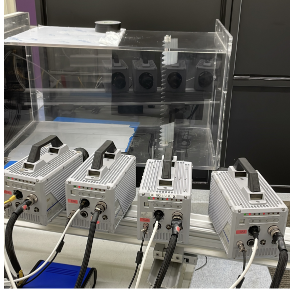
Figure 3.8: High-speed cameras arranged horizontally in a linear configuration.
