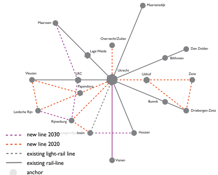
Figure 3.14: Proposed situation 2030 public transport system, schematic representation
