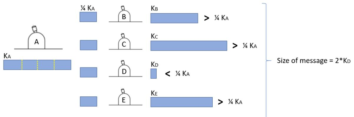
**Figure 3.4:** Diagram of the distributed message scenario. In this case, GS<sub>D</sub> limits the final size of the message.
