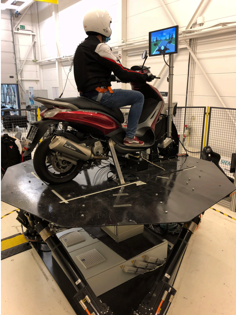
Figure 1.7: MOTORIST motorcycle riding simulator adopted in this thesis.
