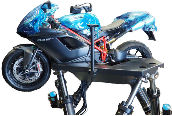
Figure 1.6: Motorcycle riding simulator developed by Cruden [155].
