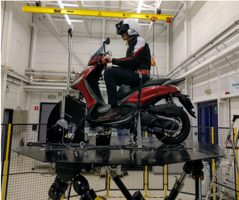
Figure 4.1: The MOTORIST simulator with a rider wearing an Oculus Rift and safety equipment.
