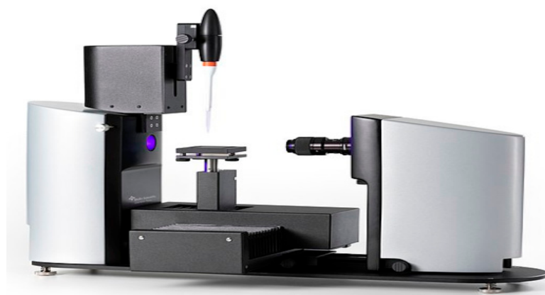
Figure 22. Measurement of contact angle using the sessile drop method.
