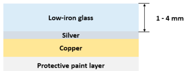
Figure 9. Second-surface silvered glass.
