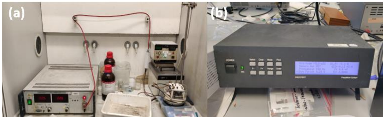
Figure 28 (a) Contact poling setup (b) Berlincourt piezometer
