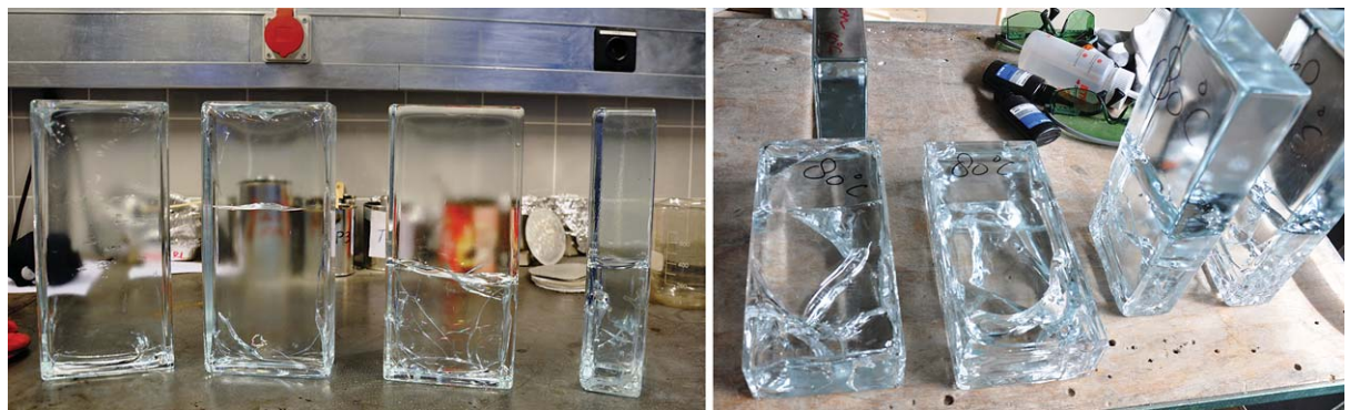
Fig. 16. Specimens A and B tested in thermal shock from 80 to 20°C. Left: Cracks in the specimens right after they were removed from the water. Right: Growth of the cracks in the same specimens the next day.
