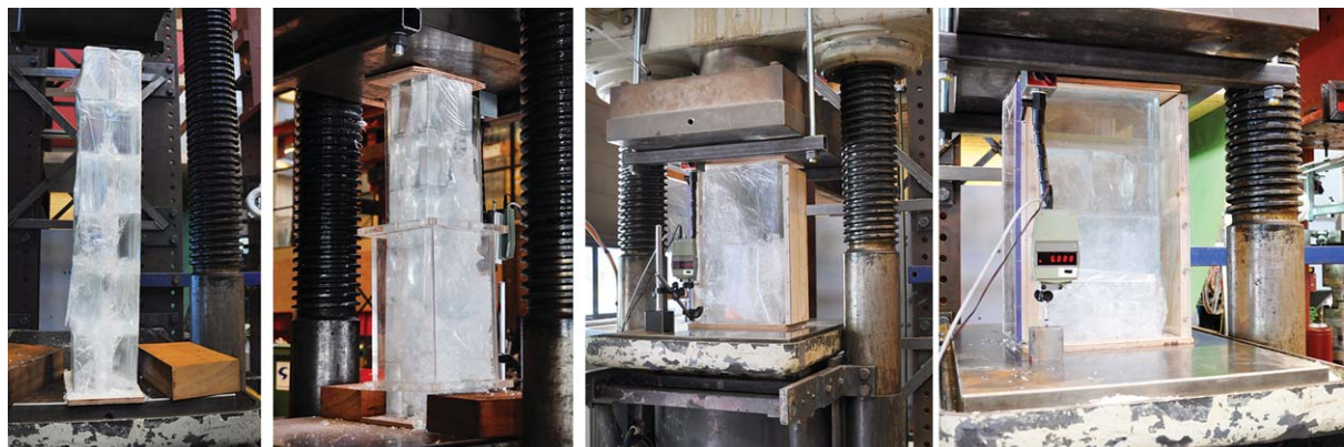
Fig. 13. Compression experiment of the columns.
