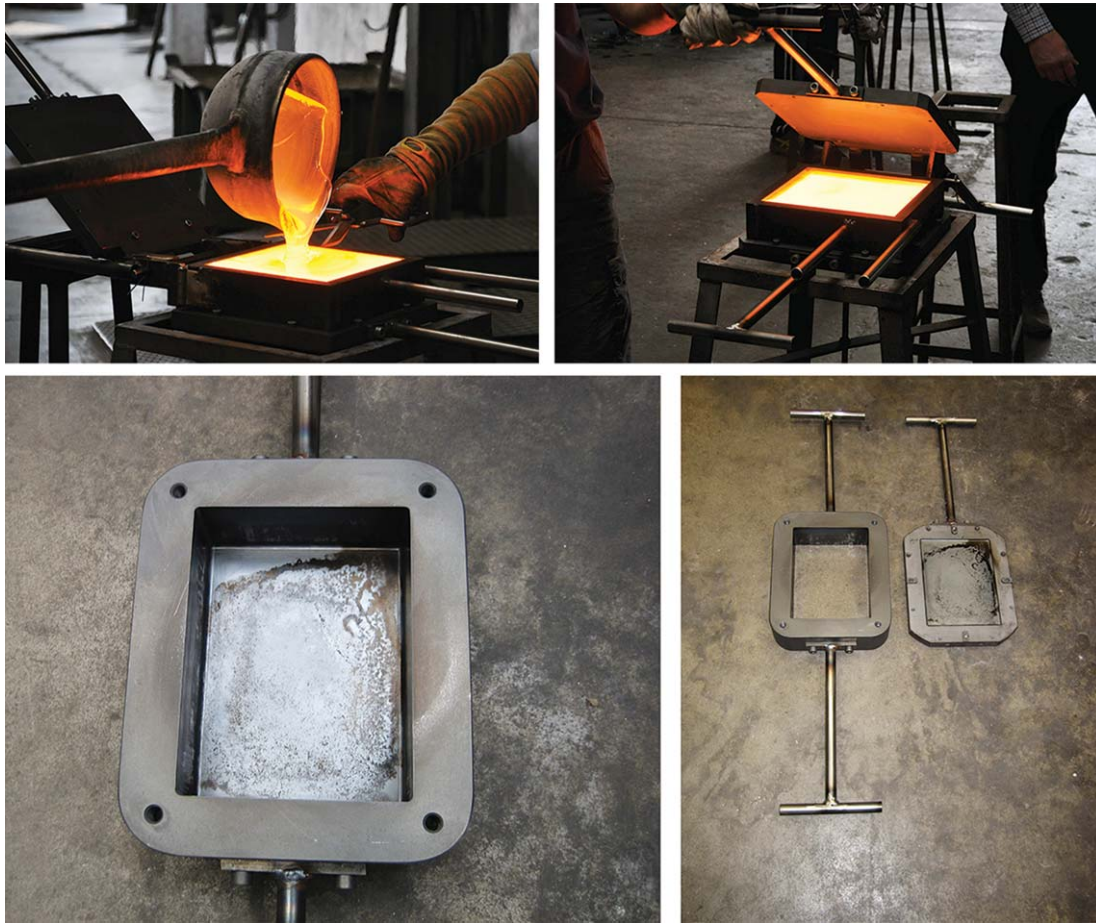
Fig. 6. Top: Casting of the soda-lime glass blocks by Poesia Company, using preliminary moulds. Bottom: Final precision moulds.
