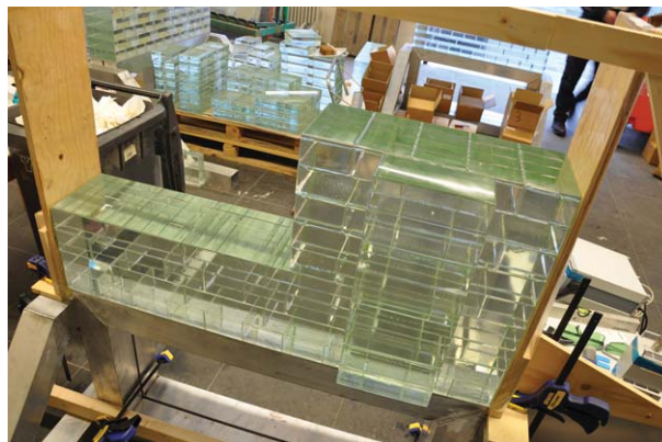
Fig. 17. Final mock up made by glass blocks with 0.25 mm precision in dimensions.
