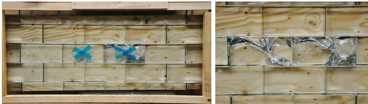
Fig. 14. Left: Results of the first vandalism test. Right: The vandalism test was then repeated to an adjacent brick. Only the aimed block was damaged.
