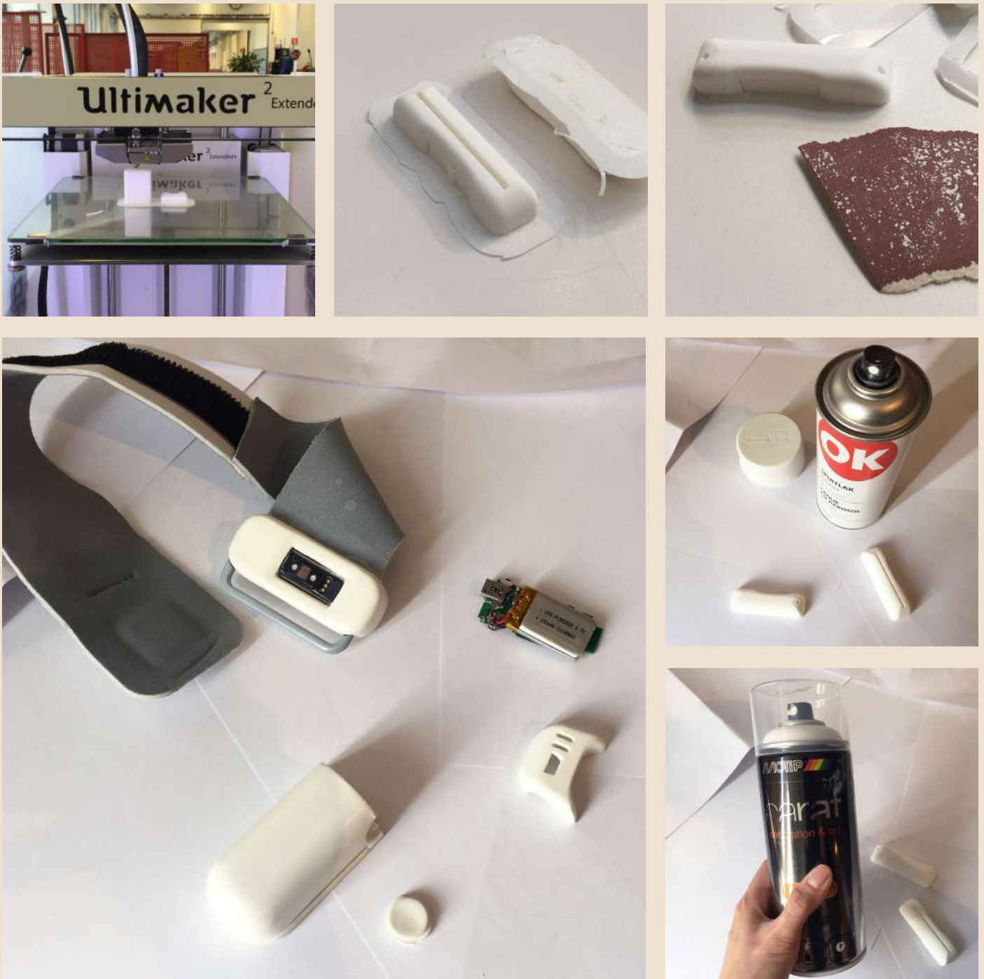
Figure 72. (clockwise from top left) 3D printing process, 3D printed parts, sanding process, spraying primer, spraying paint, printed parts
