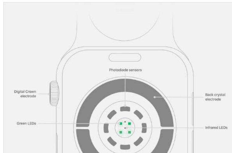
Figure 18. heart rate detection method with PPG sensor
