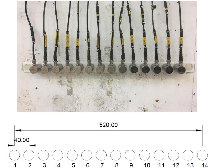
*Figure 4.4: Array arrangement: (top) in practice and (bottom) in schematic graph*
