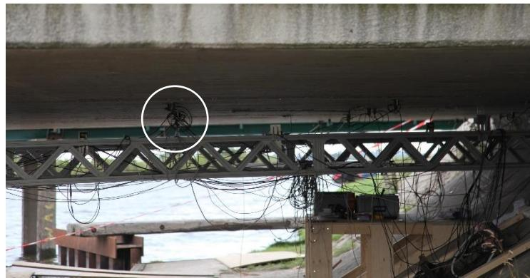
Figure 1.1: AE tests on Ruytenschildt bridge
