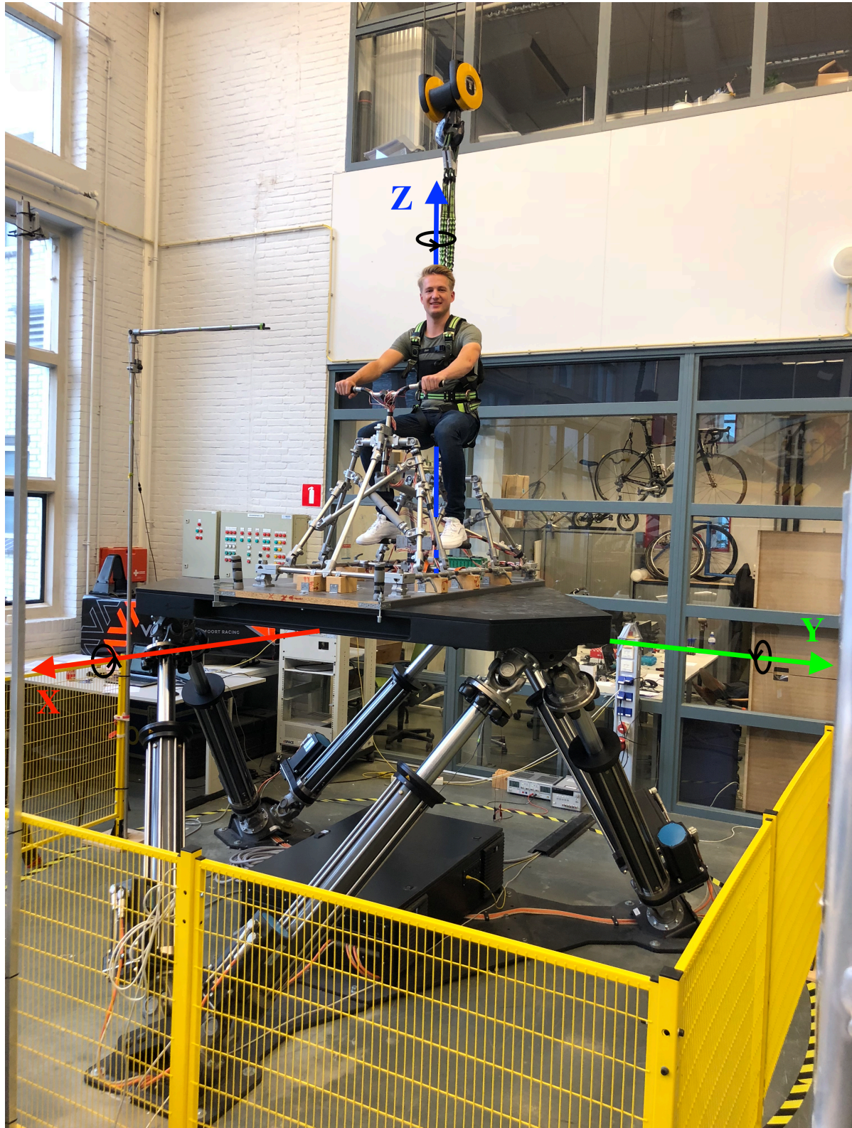
Figure 2.1: The experimental setup. Surge is the translation along the X-axis, sway is the translation along the Y-axis and heave is the translation along the Z-axis. Roll is the rotation around the X-axis, pitch is the rotation around the Y-axis and yaw is the rotation around the Z-axis. The virtual X- and Y-axis were placed 15 cm below the surface of the grey wooden base of the bicycle mock-up.
