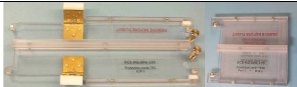
Figure 12.15: Left: cover solar cells, right: cover thin film solar cells
