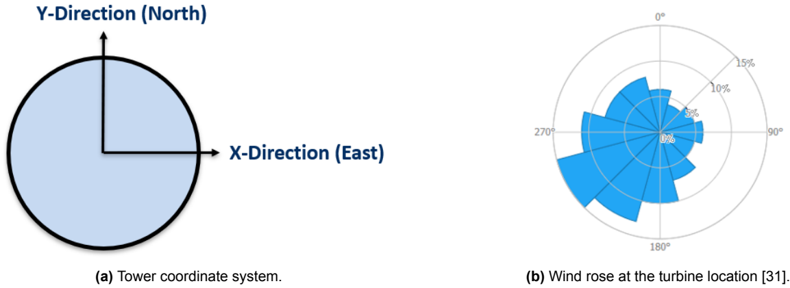
Figure 5.11: Tower coordinate convention and site wind climate.
