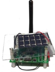
Figure 1.4: A CC2530 node powered by a solar panel and supercapacitor.
