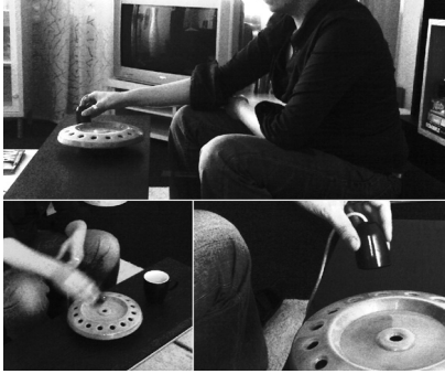
Figure 0.6. Picture of the voice mail browser. Voice mail messages are stored within one of 16 voice mail slots along its ridge and can be accessed by performing gestures above the product. The middle slot serves as a base for the input device.
