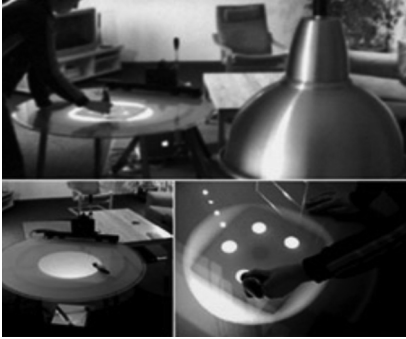
Figure 0.4. Picture of the game of pool. The pen is used to manipulate the movements of virtual balls projected on the tabletop from underneath.
