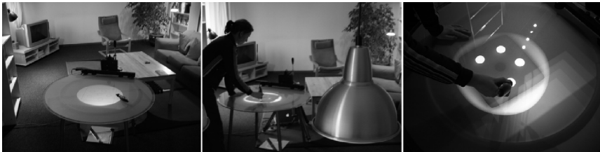
Figure 2.2. Picture of layout of the experimental setup. The interactive table is placed within a living room. The pen is used to manipulate the virtual balls projected on the tabletop.
