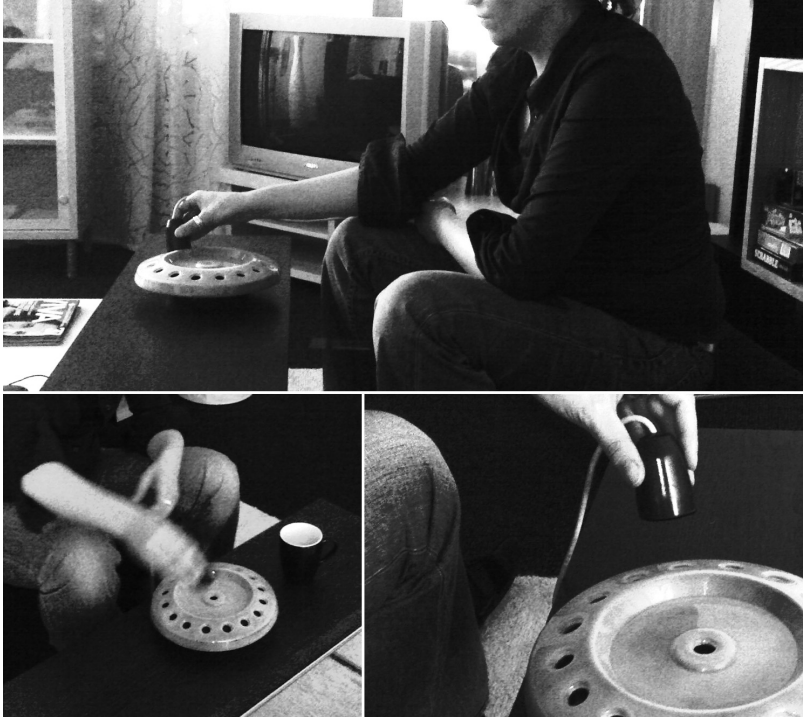
Figure 4.2. Picture of the physical product within its physical context. The physical product has a circular form, with 16 slots along the ridge and one slot within the products centre. Voice mail messages may be stored within one of the 16 voice mail slots and can be accessed by performing gestures above the product. The middle slot serves as a base for the input device.
