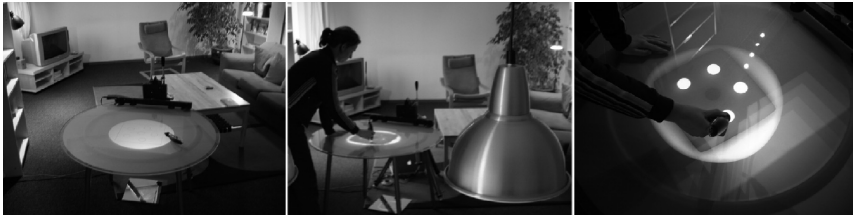
Figure 1.2. Picture of layout of the experimental setup. The interactive table is placed within a living room. The pen is used to manipulate the virtual objects projected on the tabletop.
