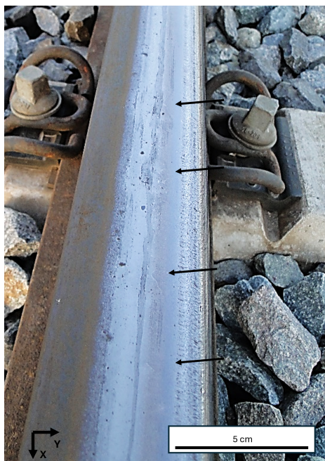
Figure A.3: Running surface of the rail made from rail steel with improved wear properties. The arrows indicate the squat-type defects that are present. Defects cause only minor subsidence of the surface which is typical for rails made from these steels.
